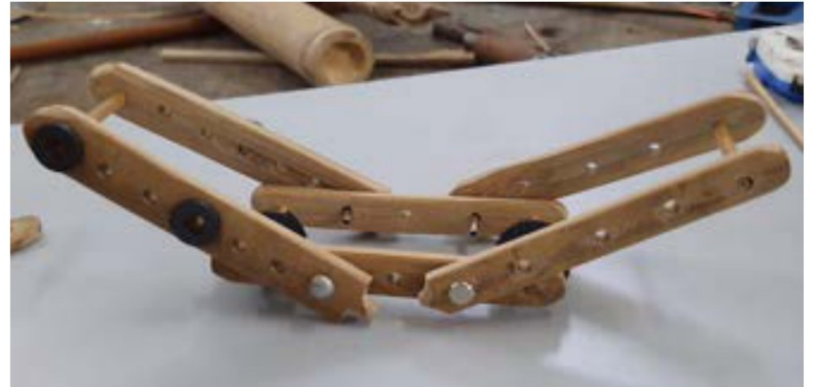
Rivets and screws were used for connection
