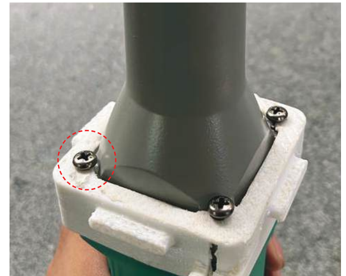
Fig 23.2.3: User Test For Clamping By Existing Screws
