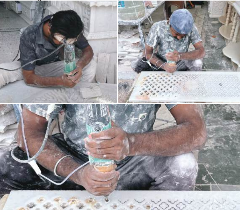
Fig 15.2.2: Machine Held Straight 90 Degrees
