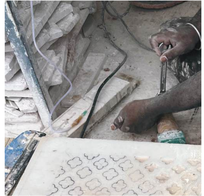
Fig 23.5.3: Observation For Bit Replacement
