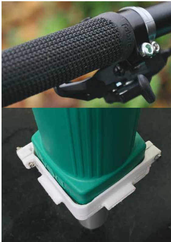
Fig 20.1.2: Two Additional Screws To Clamp
