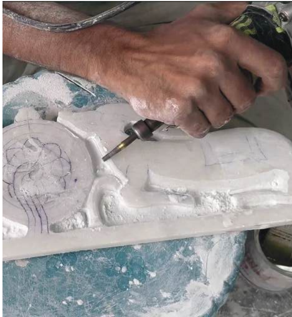
Fig 15.5.1:Dust Emmission When Machine Angled
