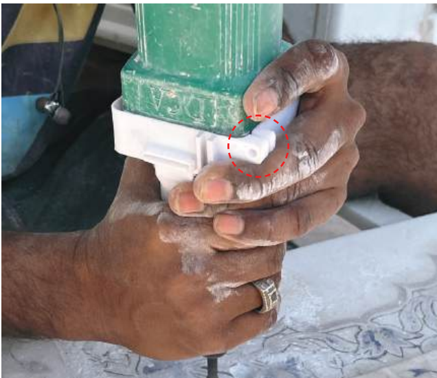
Fig 23.2.1: User Test For Clamping By 2 Side Screws
