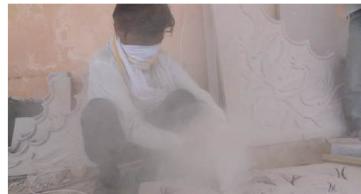
Fig 12.1: Dust Emission While Stone Cutting
