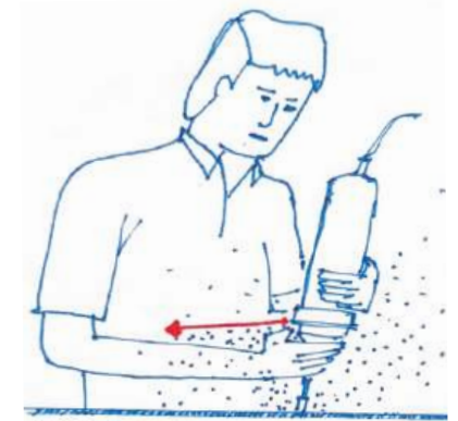
Fig 20.11.2: Diverting Existing Vent Towards One Direction
