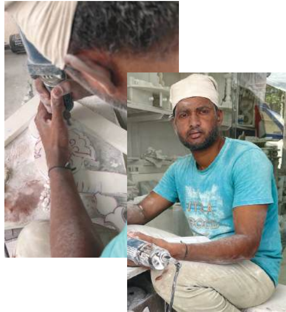
Fig 15.5.2:Dust Emmission With No Water Supply
