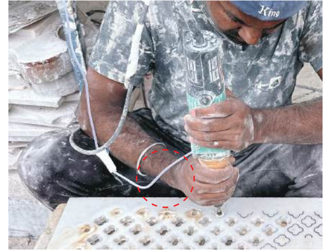
Fig 20.7.3: Issue of Pipe Falling On Hand
