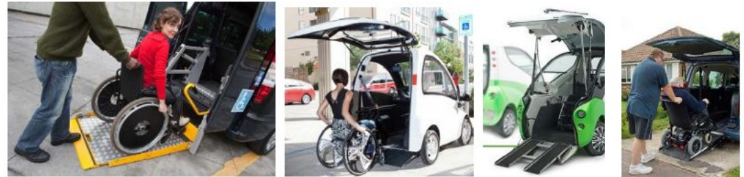
Fig 42: Hydraulic lift for wheelchair, Ramp
