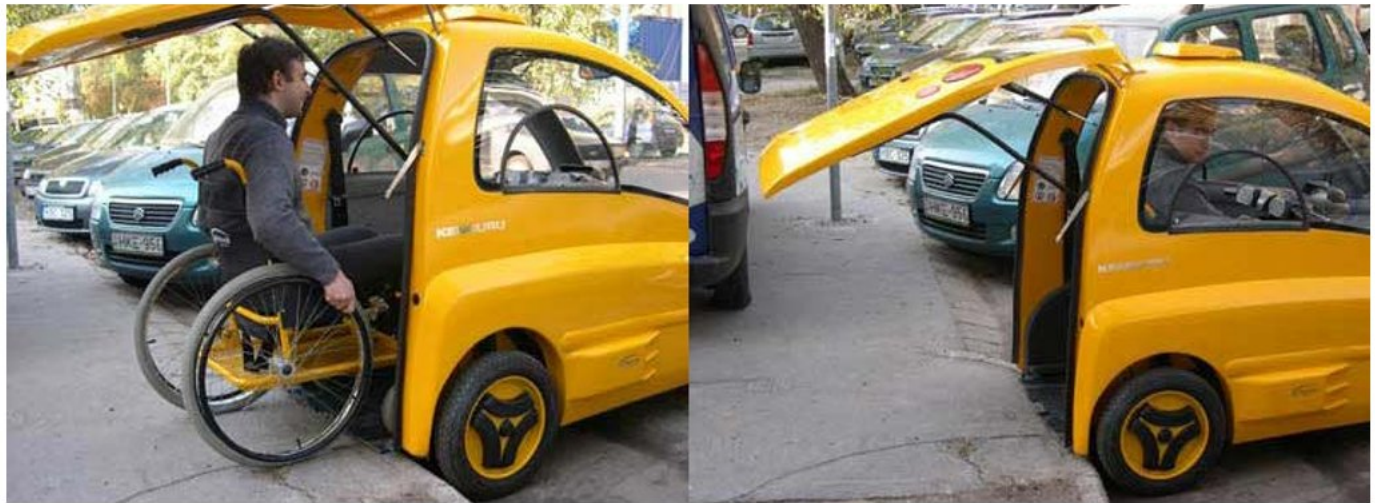
Fig 26: Kenguru has an automatically lowering ramp, which comes down as the back door opens, using remote control
