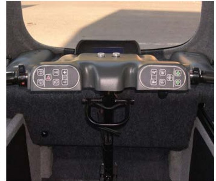
Fig 28: Kenguru features motorcycle type handlebar controls
