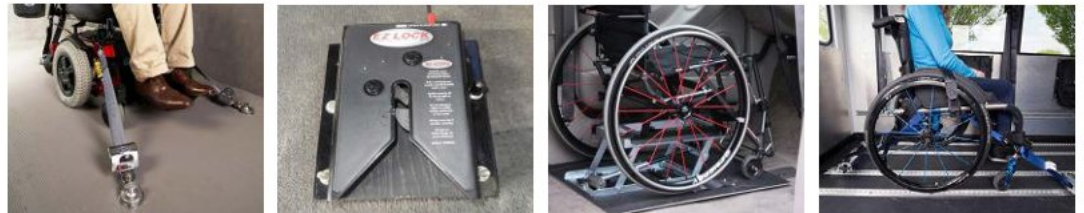
Fig 45: wheelchair locking system, EZ locks
