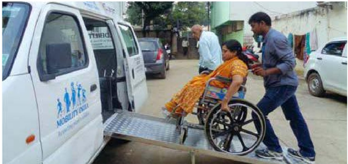
Fig 20: Side Entry for wheelchair users
