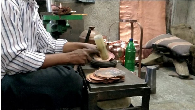
Shaping of sheets of copper to desired shapes by hammering
