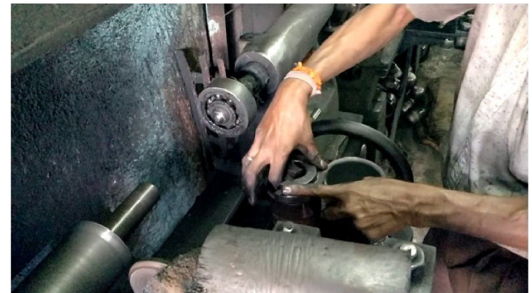
Split die being used as a guide for the form of the utensil
