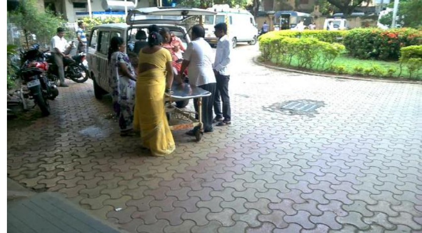
Smaller omni cannot house a fully foldable stretcher, making it difficult to unload and transfer the patient
