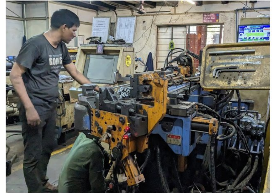
CNC bending atPanchal Automobiles
