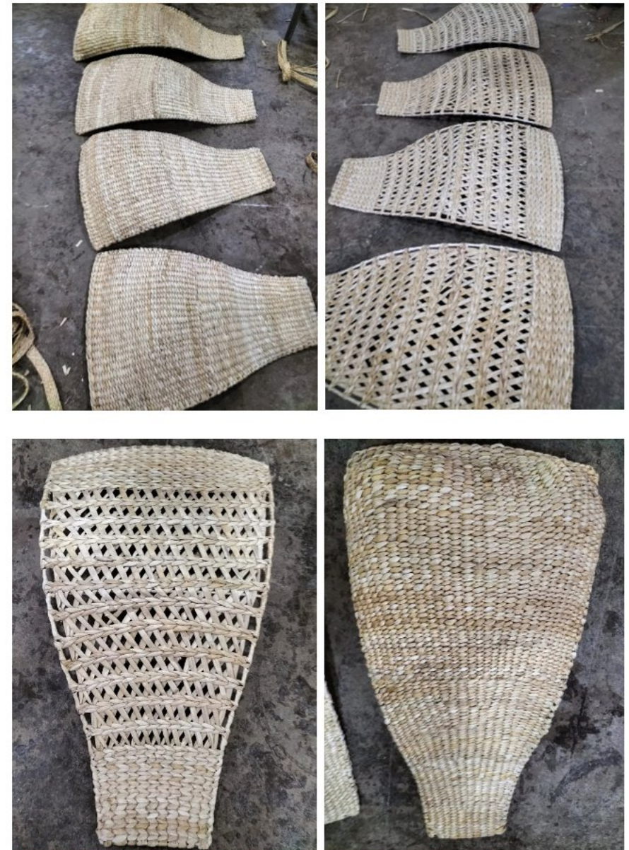
Weaving over the metal frame with ropes or narrow sheaths
