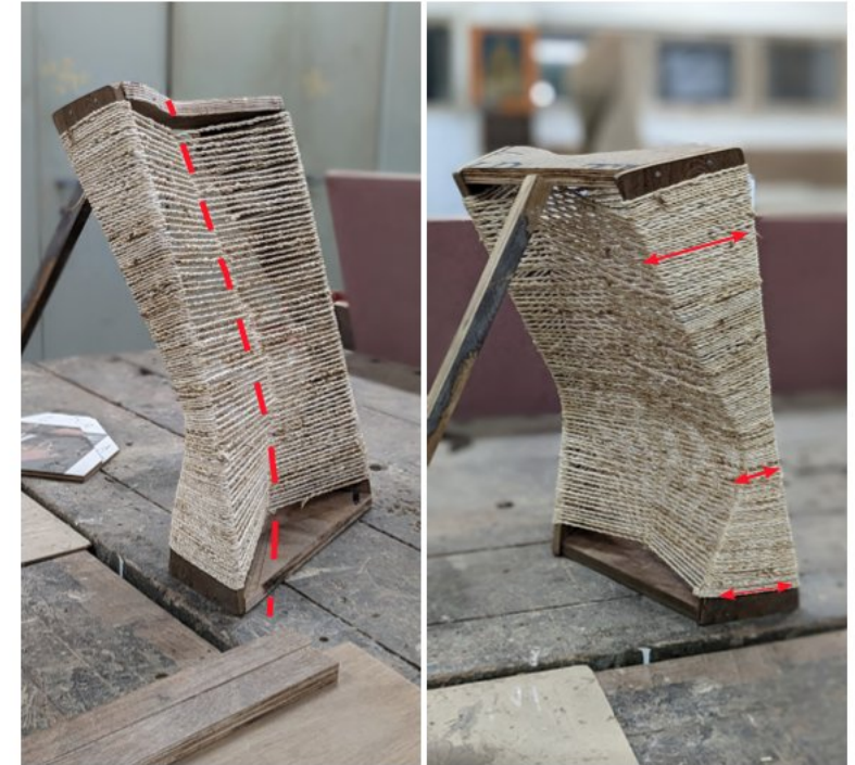
The design of this backrest is based on the Concept 3 of the Ideation where the ropes are winded criss cross along the frame to form a central intersection line which adapts the human lumbar support.
