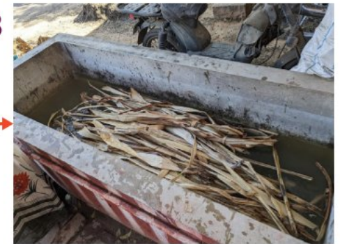
3 Wetting Process before fibre separation
