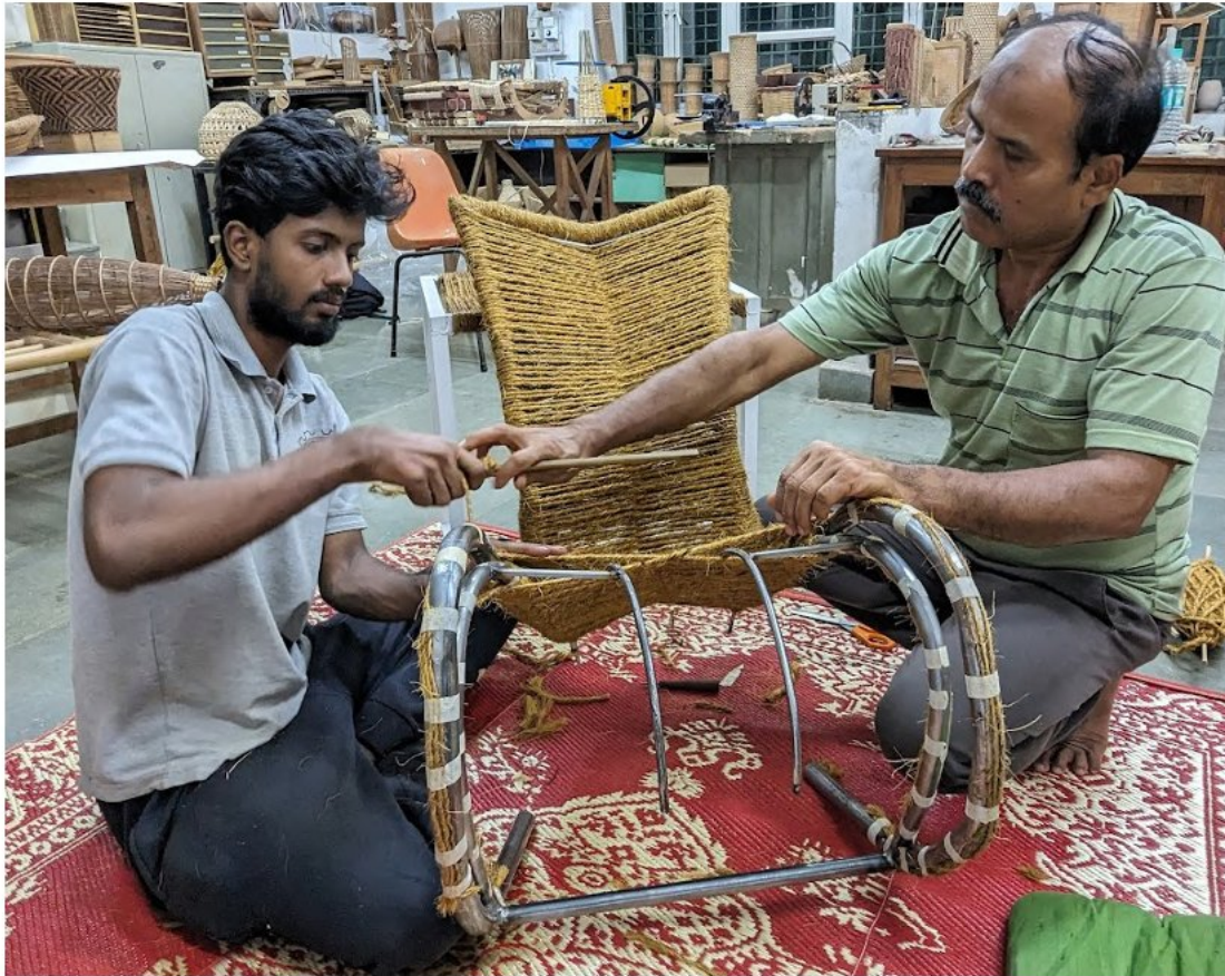
Criss - cross weaving with fiber ropes
