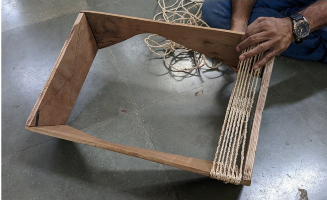
Backrest module made with plywood frame having the variable side widths to adapt the ergonomic form
