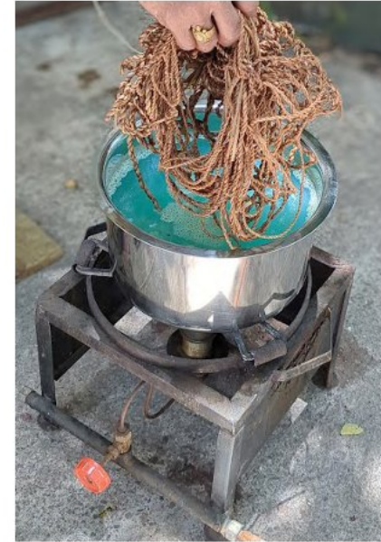
Boiling with Copper sulphate
