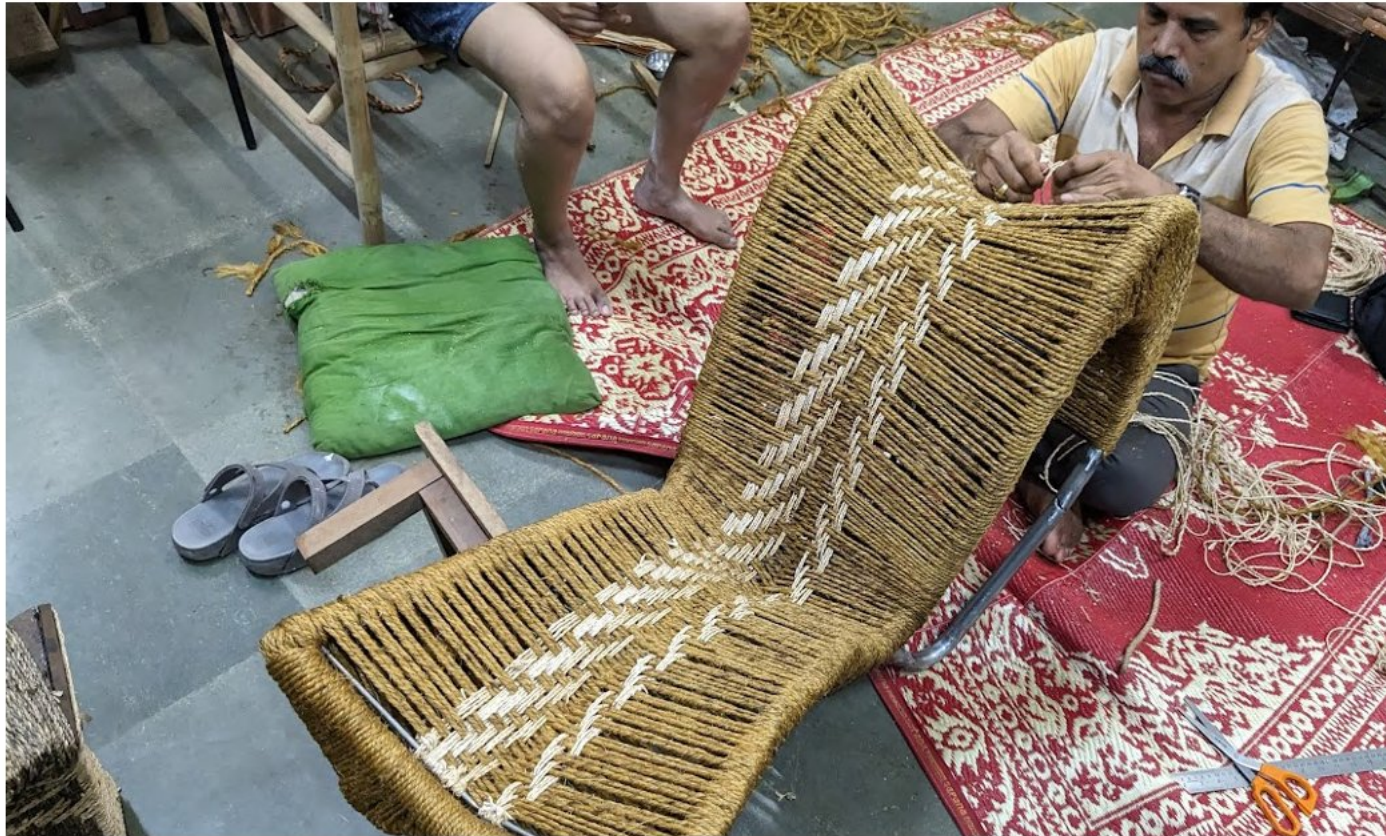
Weaving vertically with Banana stem ropes
