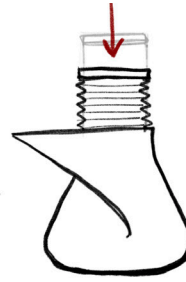
Bellow added to suggest pushing down. motion inspired from french press and areo press
