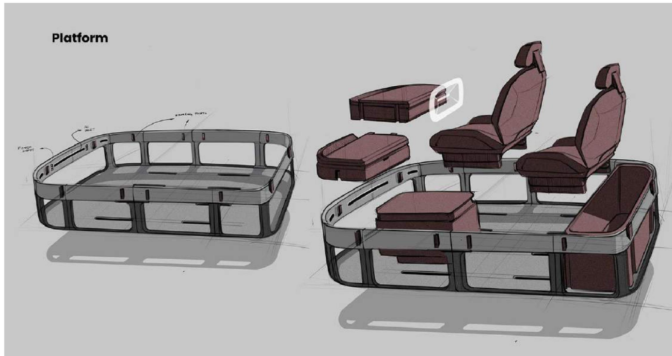
Fig. 13.1 Concept sketch of the modular platform for interior
