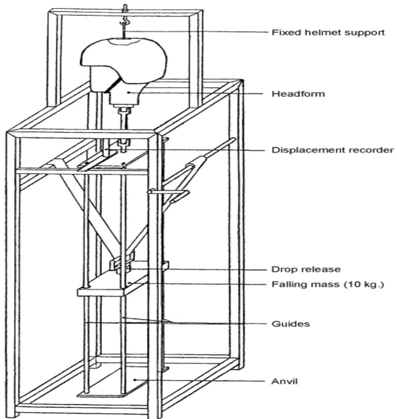
**Fig. 1 DYNAMIC TEST OF RETENTION SYSTEM**
