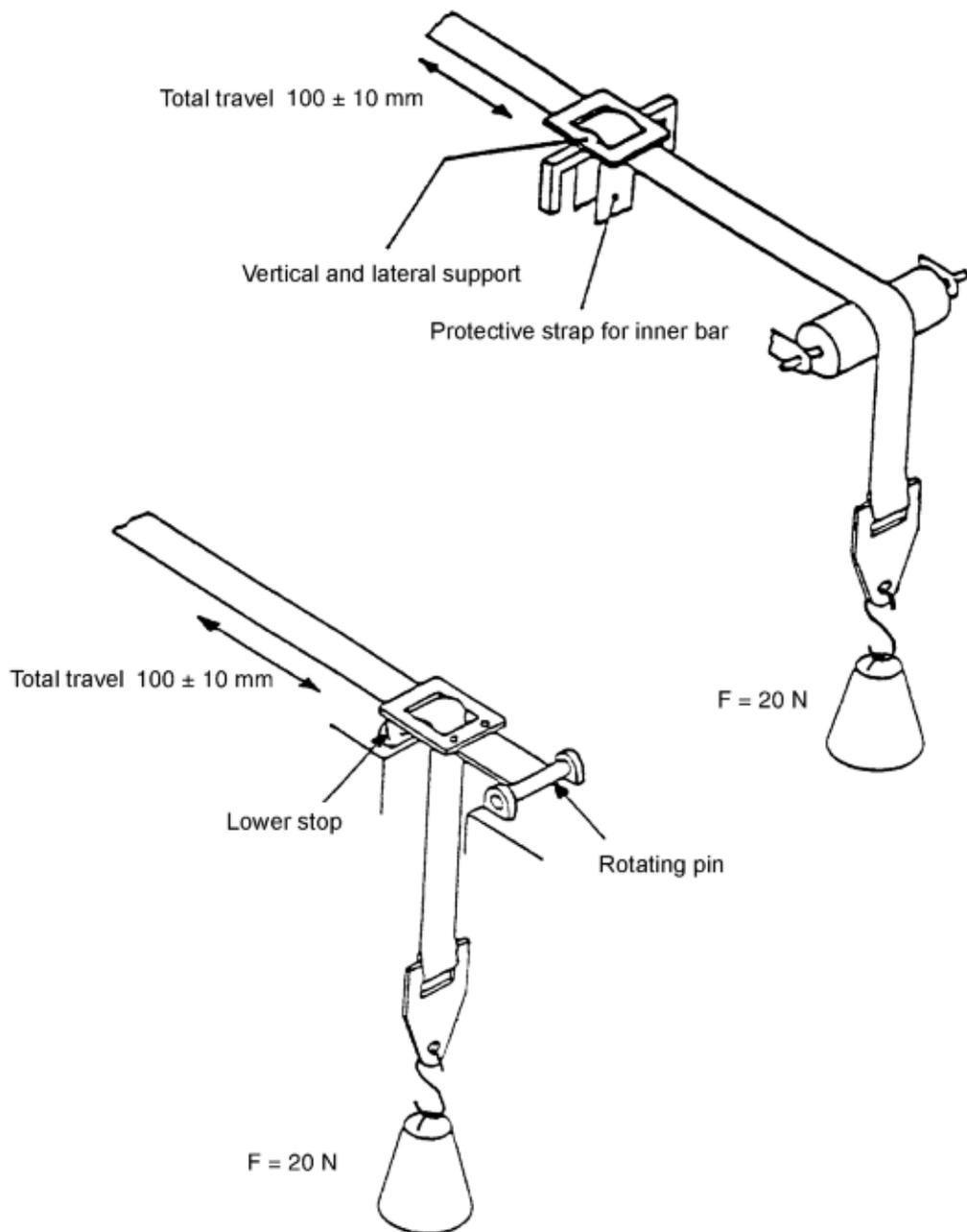
**Fig. 2 APPARATUS FOR TESTING ABRASION OF THE CHIN STRAP**
