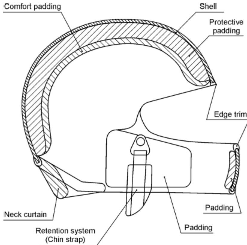
Fig 1 TYPICAL SKETCH SHOWING INTERNAL COMPONENTS OF HELMET
