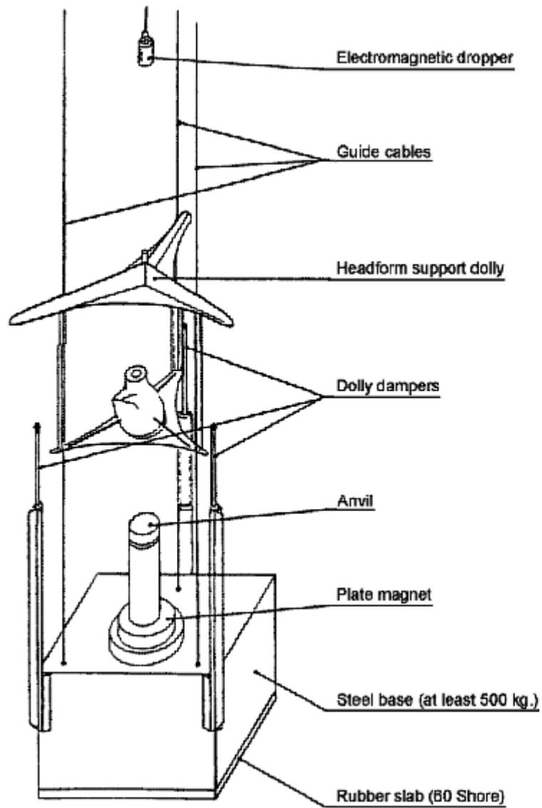
**Fig. 1 TEST MACHINE HEADFORM DROP ASSEMBLY**
