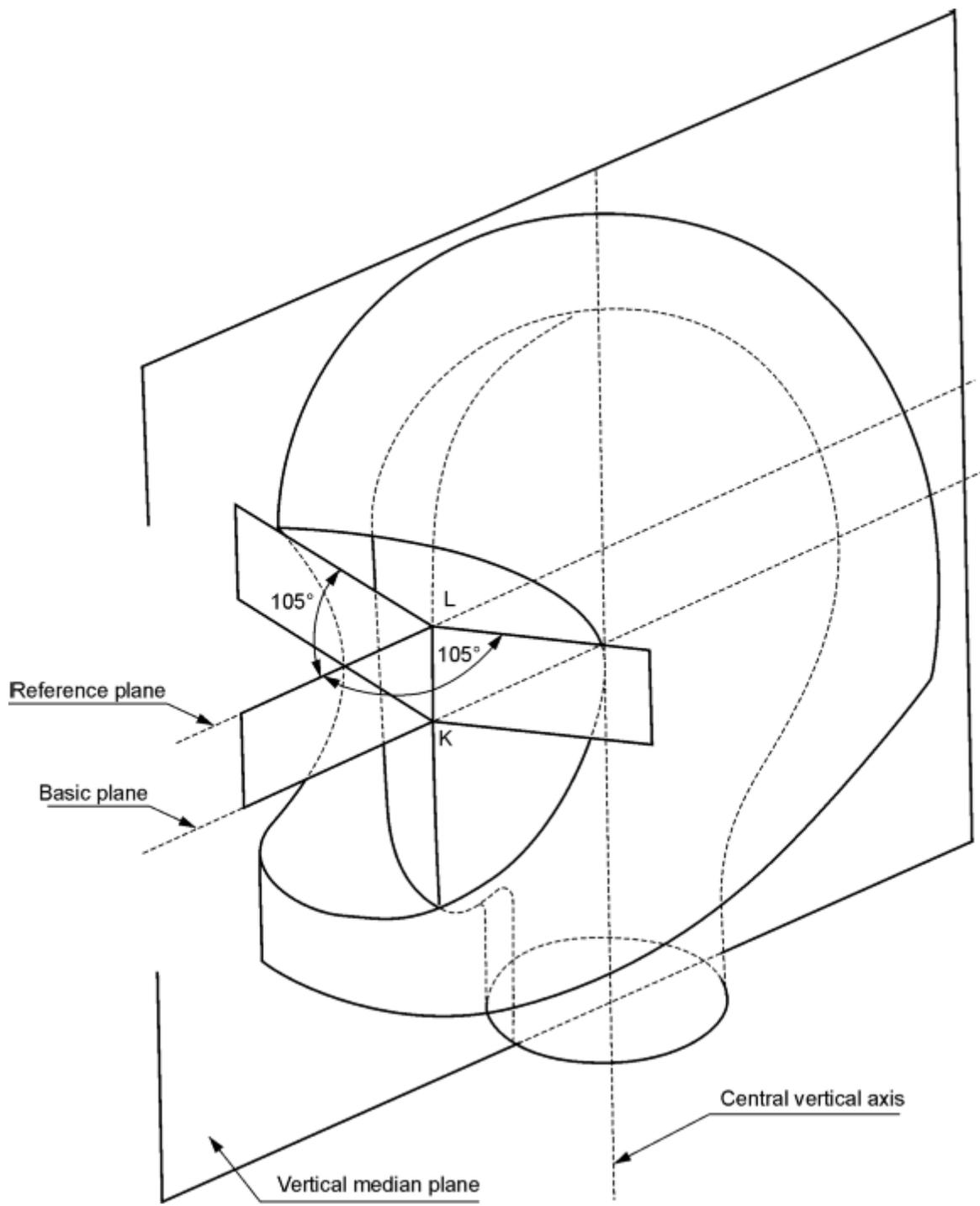
**Fig. 2C PERIPHERAL VISION – HORIZONTAL FIELD**
