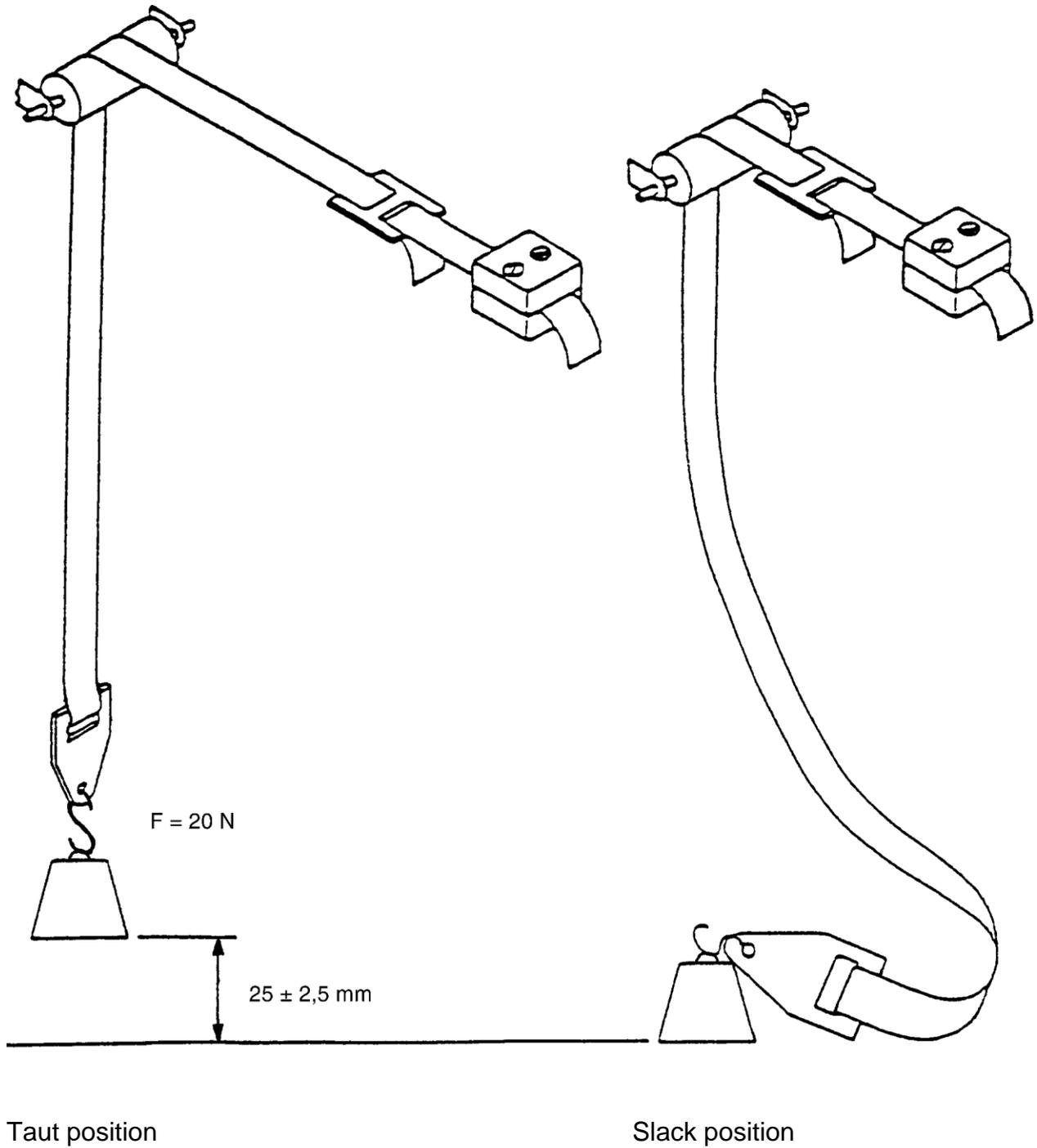
**Fig. 1 APPARATUS FOR TESTING SLIPPAGE OF THE CHINSTRAP**
