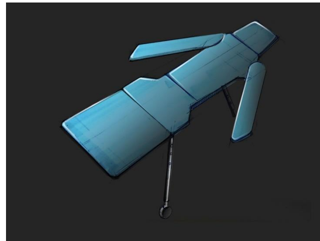
(Fig:7.7d) the arms of the table can be extended out for better accessibility for connecting intravenous tubes during surgery.
