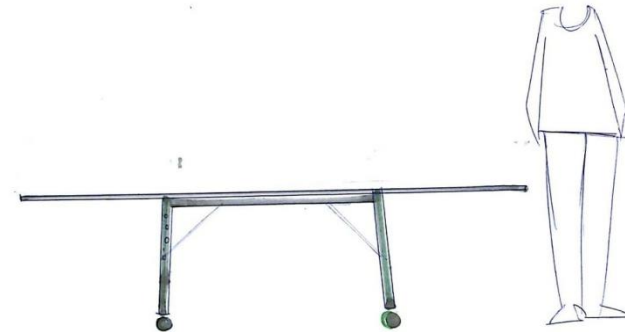
(Fig:7.7b) OR table lowered by retracting the telescopic legs
