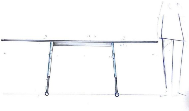
(Fig:7.7a) For adjusting height the telescopic legs are extended
