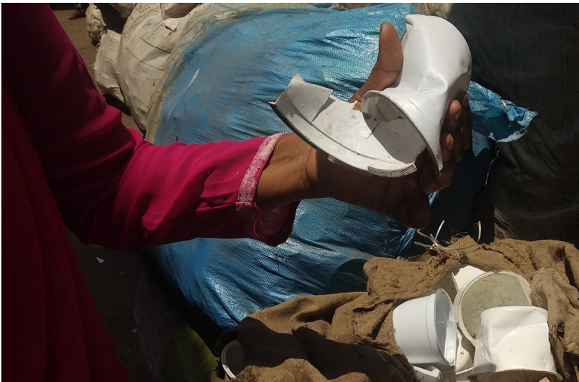
Image 6.4 If the plastic is not sorted terms of colour, the end product may turn out to be grey in colour when the plastic is melted and reformed during recycling process
