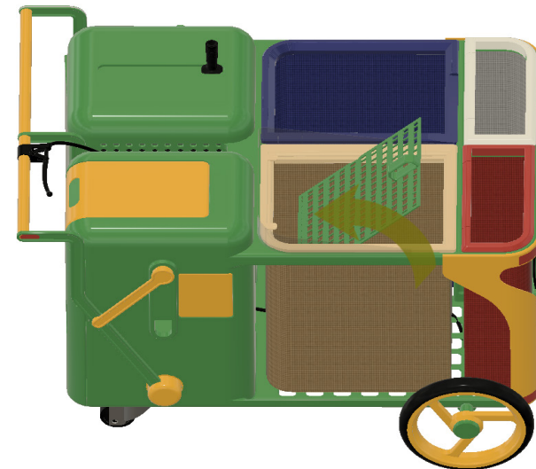
Step 4- The mesh tilts thus transferring the inert waste into inert compartment
