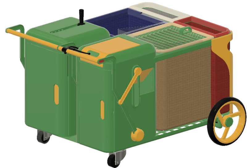
Step 2- The lid is tilt-able and can easily let through a 2 liter PET bottle
