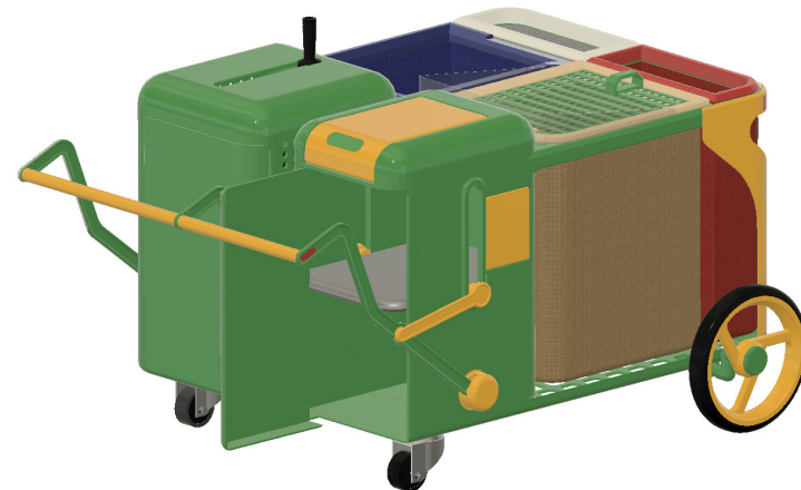
Step 4- This action compresses the plastic bottles. The torsional spring brings back the rod into its original state
