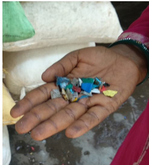
Image 6.5 The sorted plastic is shredded in pieces for further recycling process
