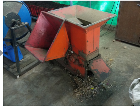
Image 3.9.3 A shredding machine is used later to shred the waste
