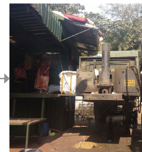
Image 3.3.9 Wet waste is compressed by the hydraulic garbage compactor. Dry waste is partially recycled
