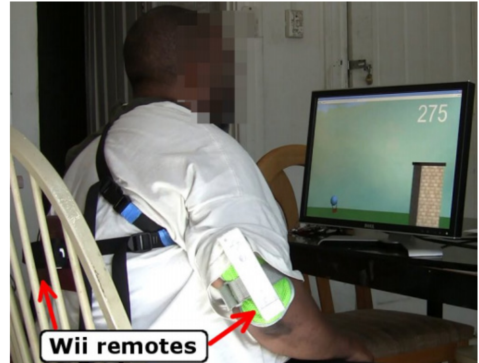
Figure 3.9 - Participant playing the game with multiple Wii remotes strapped to arm and back to detect compensatory motion.
