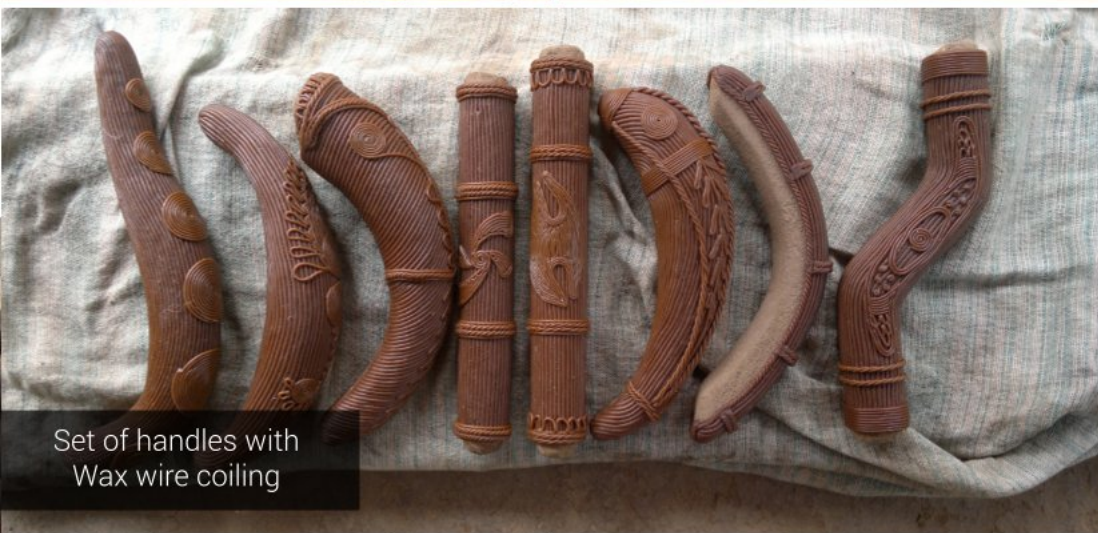
Wax coiling on clay core
