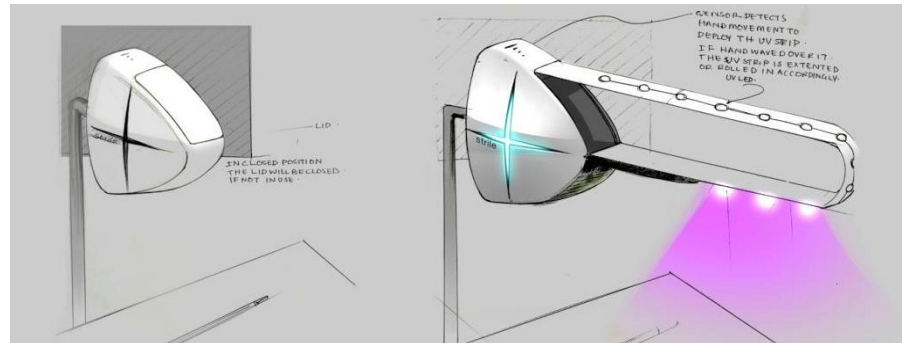
Fig:10,2d when not in use the LED strip is retracted
