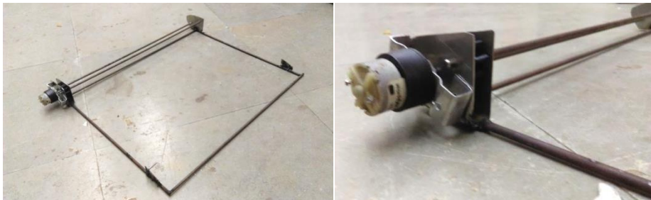
Fig:10,.1c The lid opening mechanism assembly.
