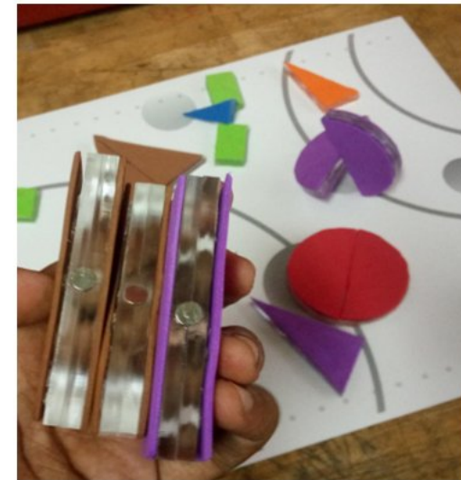
Figure 42: Blocks with magnets inlay for joining
