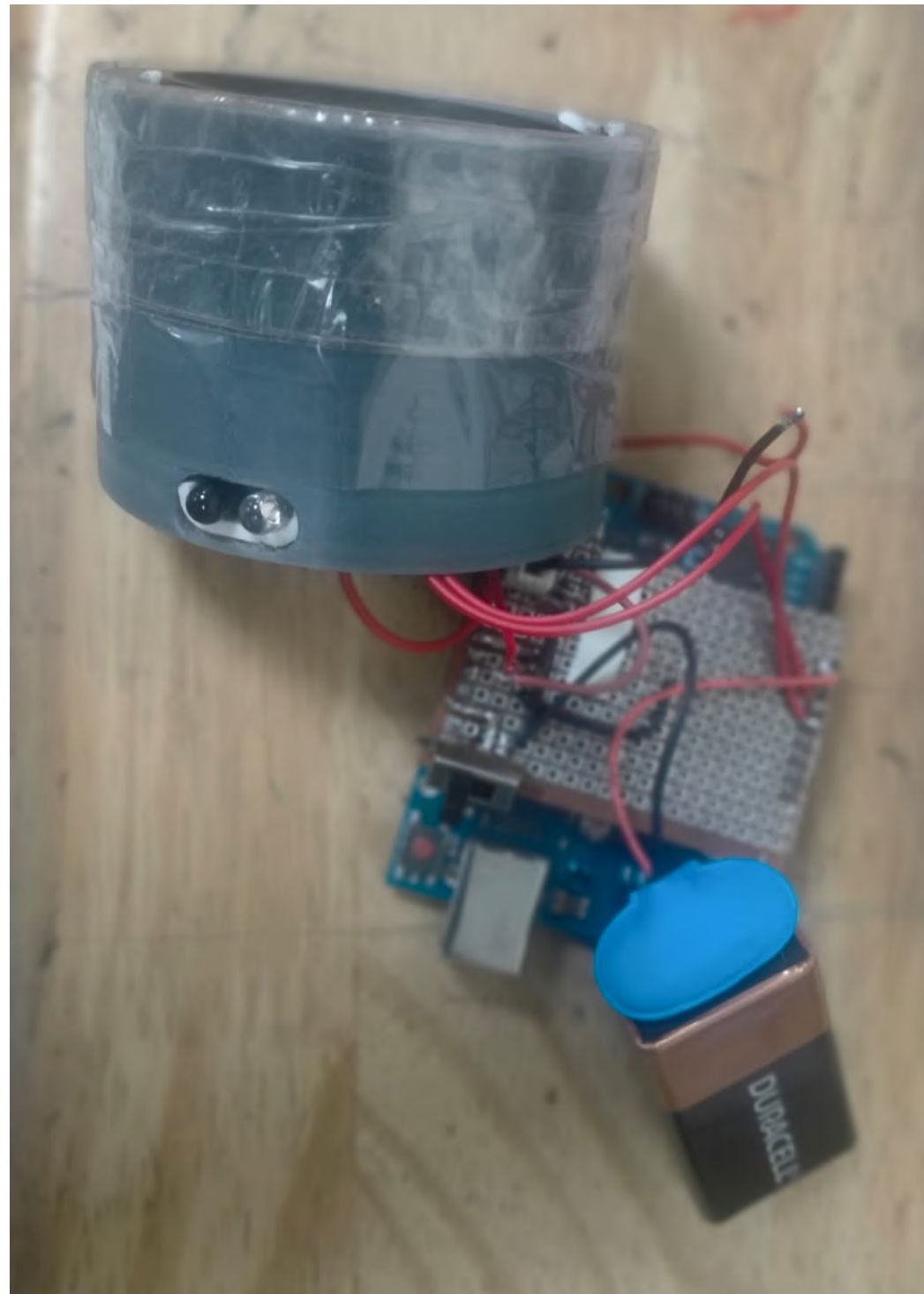
Fig. 38 Initial set-up which used an Arduino Uno, was later switched to an Arduino Nano in order to make the circuit more compact
