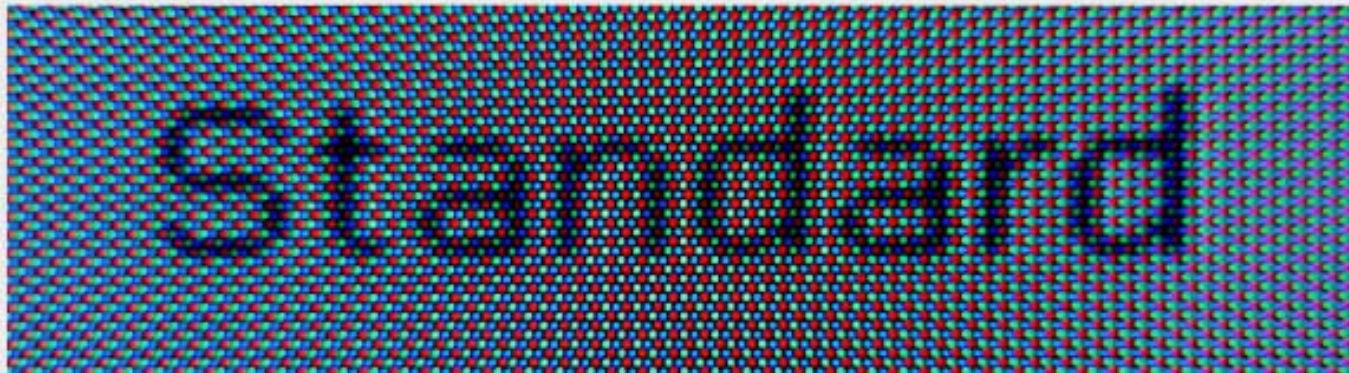
Pixels and Text on a CRT Computer Monitor
