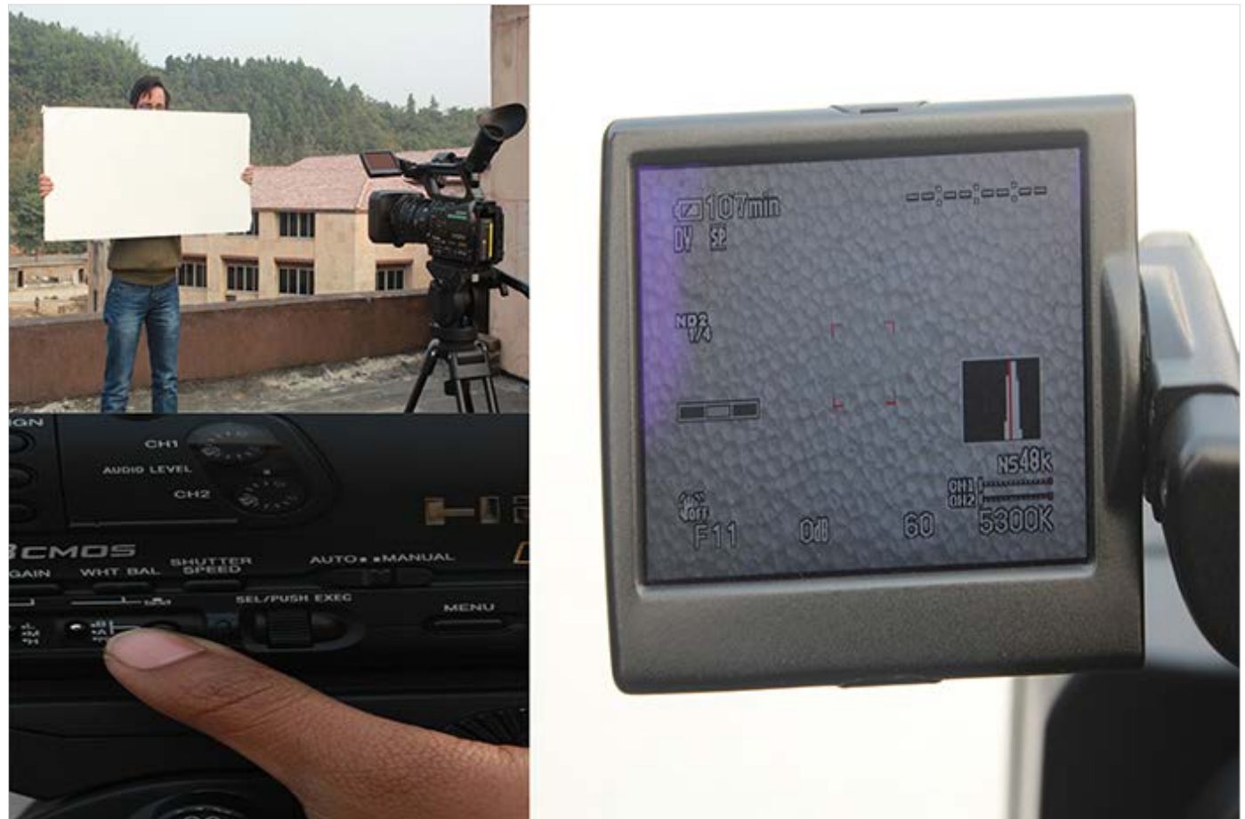
Fig.7: Color Temperature - Auto White Balance adjustment in an EFP camera.
