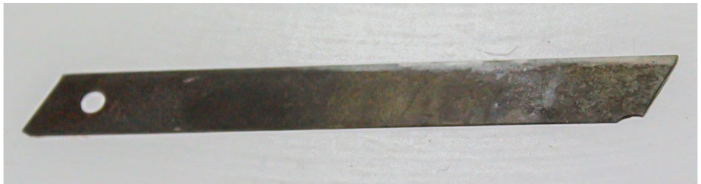
A piece of the blade is used to cut and shape the clay as per requirement.
