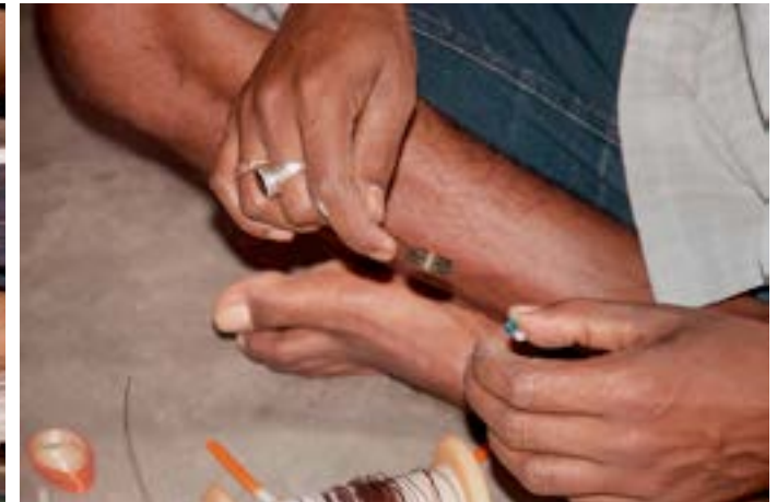
Artisan combines copper wire with beads and put it into a ring-shaped bamboo strip.
