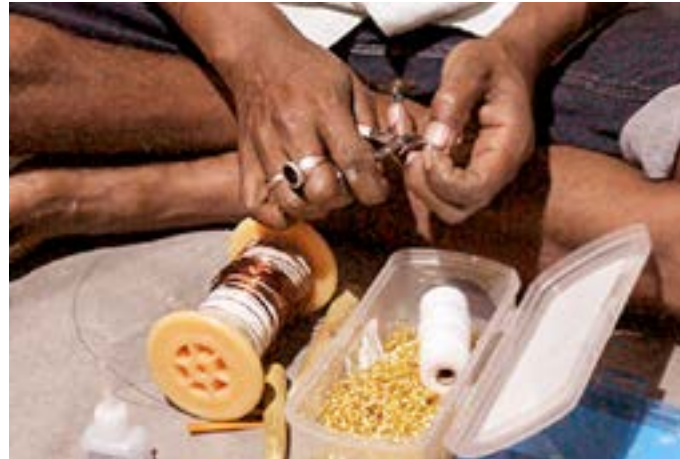
Artisan is cutting the copper wire with a flush cutter tool.
