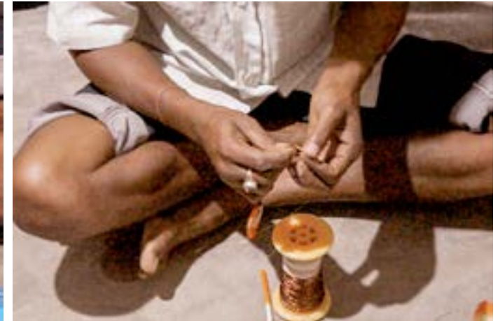
Inserting the copper wire in a bamboo strip ring.
