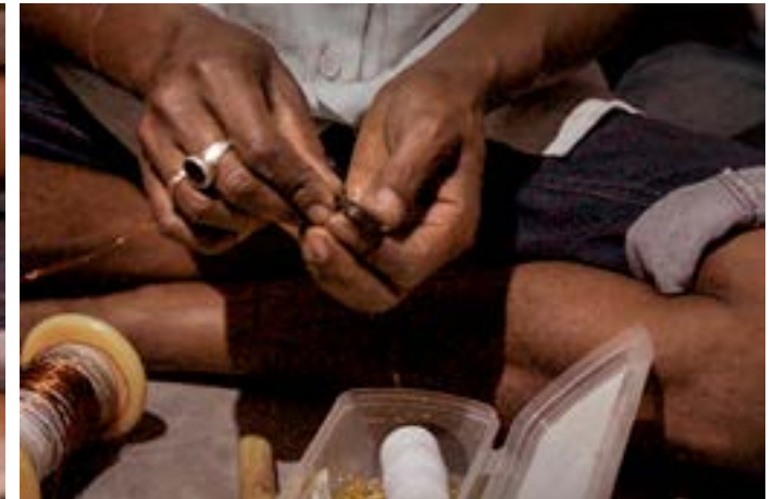
The artisan makes the hole on the bamboo strip for inserting the copper wire.
