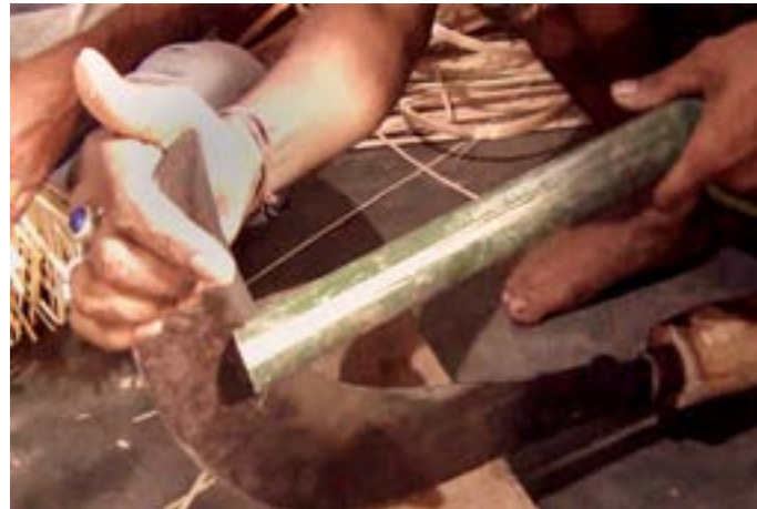
Customized knife tool used to cut the bamboo.
