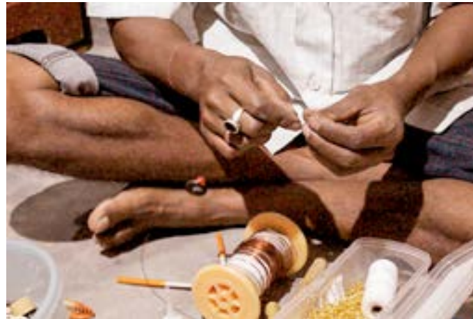
Inserting the copper wire in a bamboo strip ring.
