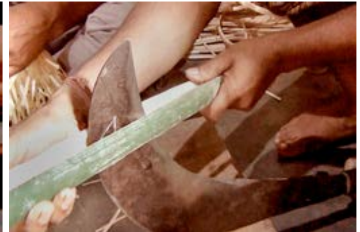
Artisan divided the bamboo into two half with the customized tool.
