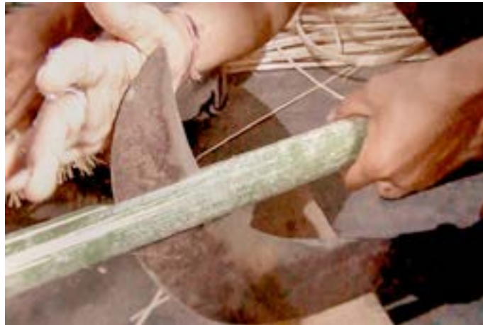
Artisan divided the bamboo into two half with the customized tool.
