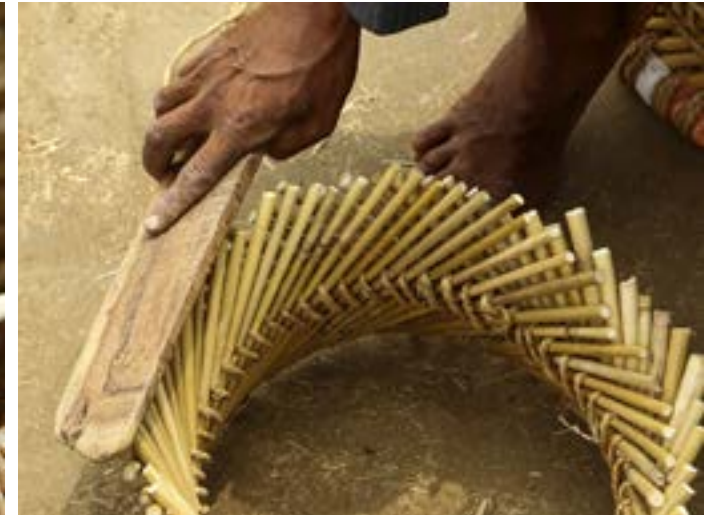
Flat Wooden piece known as Thokni is used to beat the bamboo.
