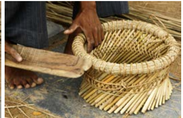
Prepared base is beaten with a flat wooden piece (thokni) to settle the loops.
