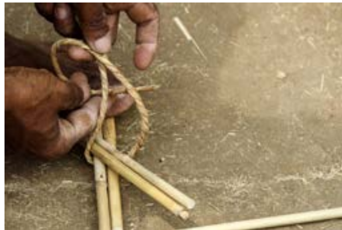
Pairs of bamboo sticks are arranged opposite each other in criss cross manner.
