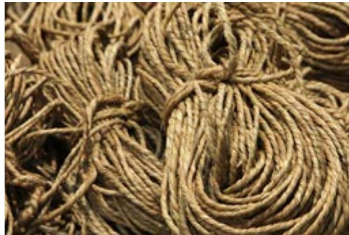
Twines made out of bamboo waste.
