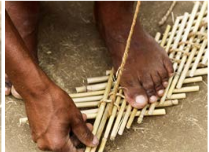
Bamboo straps are weaved till the required length.
