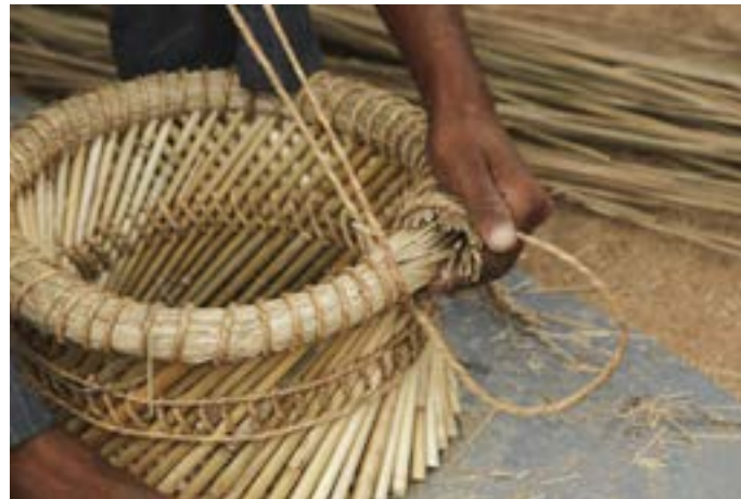
Ends of thush are inserted and tied firmly with twine.
