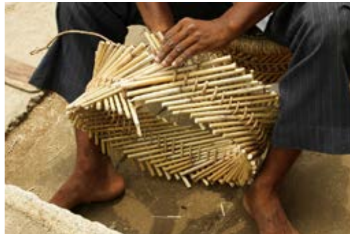
Prepared strap is then rolled into a circular form.
