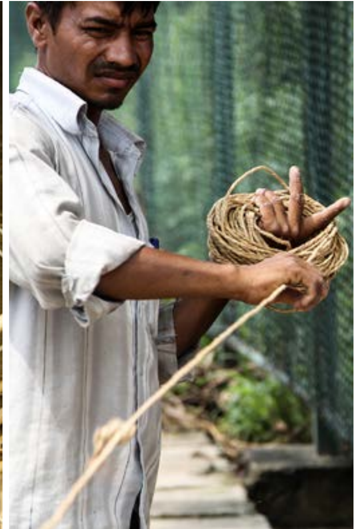
The wasted strips are taken and twisted into bamboo twines.
