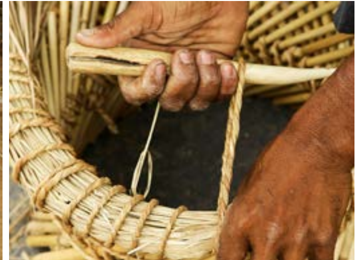
With a small wooden hook (Singri) the twines are pulled to tighten the loops.
