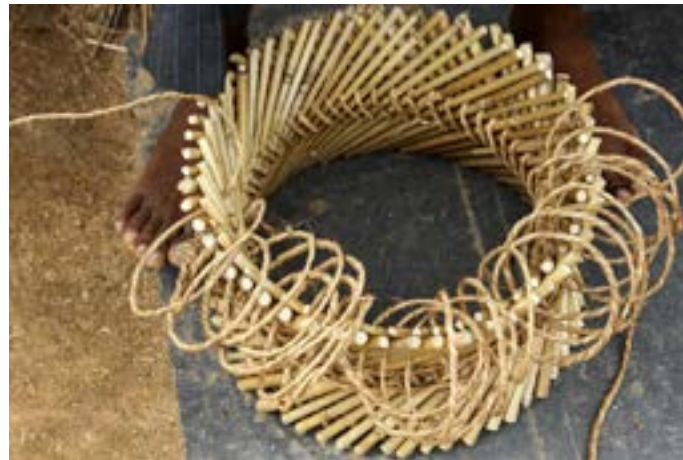
Loops of twine are made around the bamboo strap.
