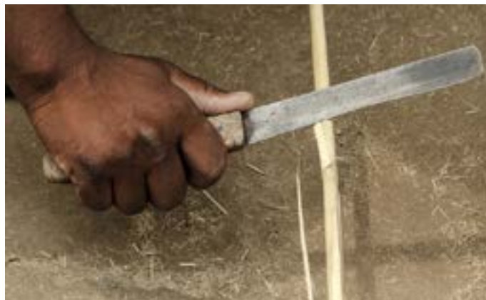
Thin strips of bamboo are cut using a knife.
