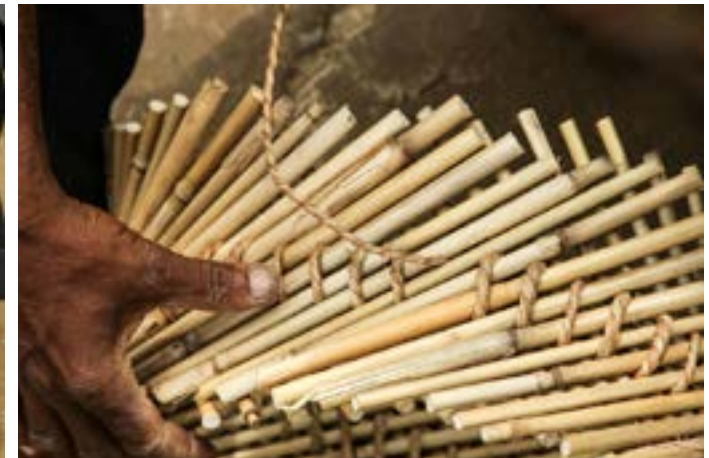
The ends are tied and knotted with bamboo twine.
