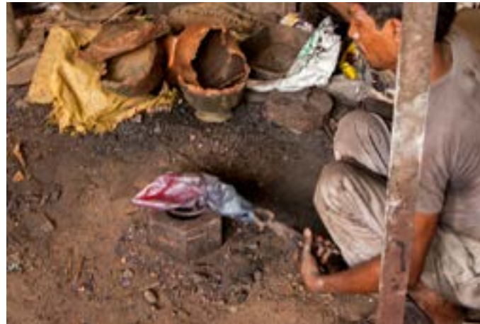
Crushing the old brass metal using hammer to recycle the metal.
