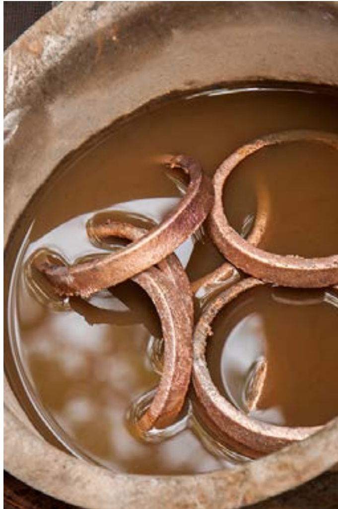
The solidified castings are placed in cold water for cooling.
