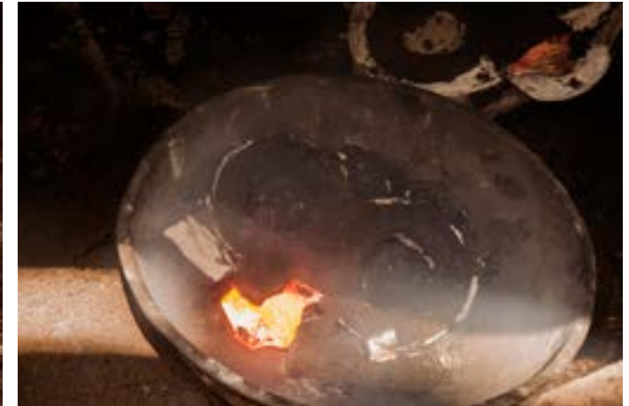
The castings are separated from mold by using pincer.
