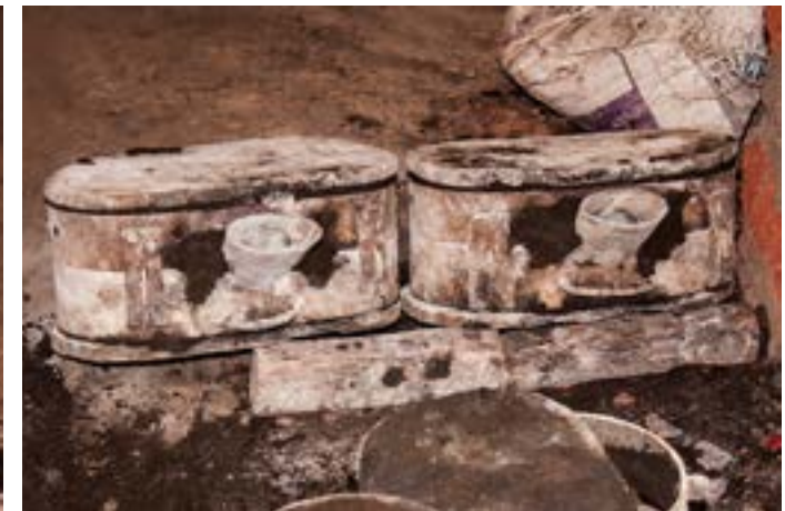
Finally molds are ready for casting.
