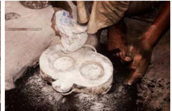
Chalk powder is sprinkled on top of the design so that the soil mixture doesn't hold onto it.
