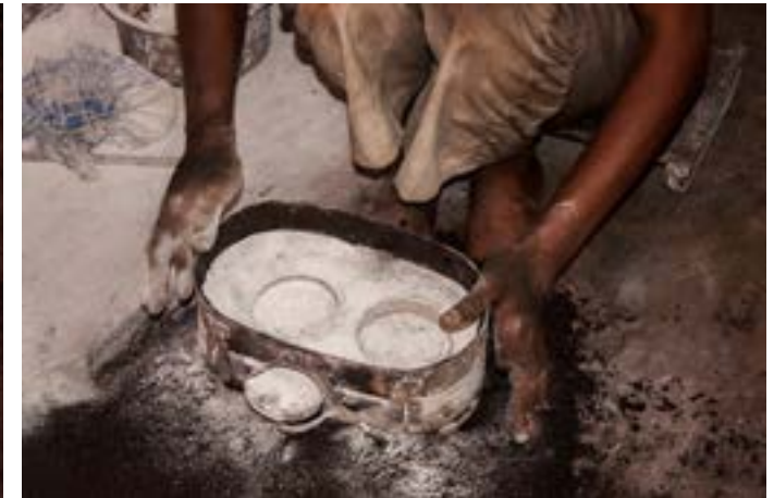
The mold frame is placed on the wooden plank.
