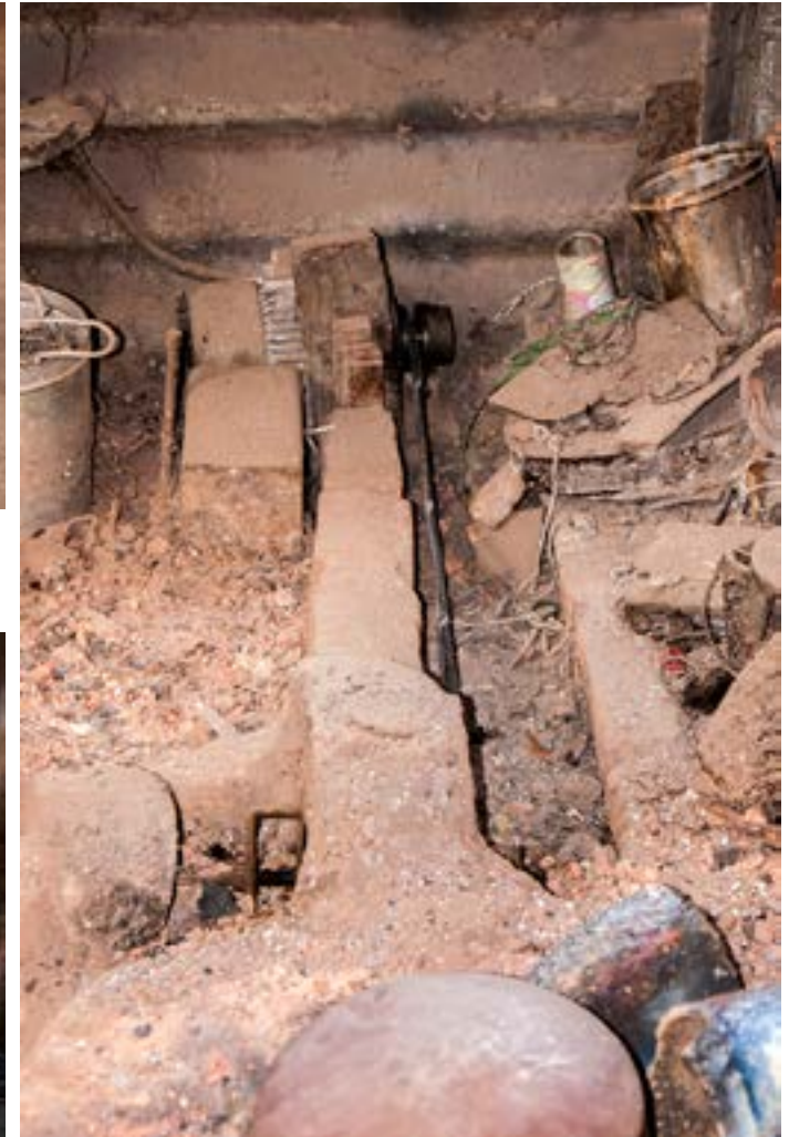
Electric air blower used to blow the air to custom made furnace.
