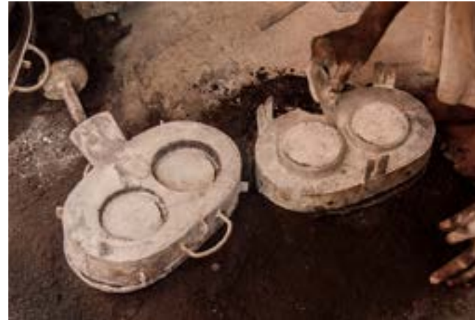
Making a pathway for the molten metal to pass by using custom made cutter.
