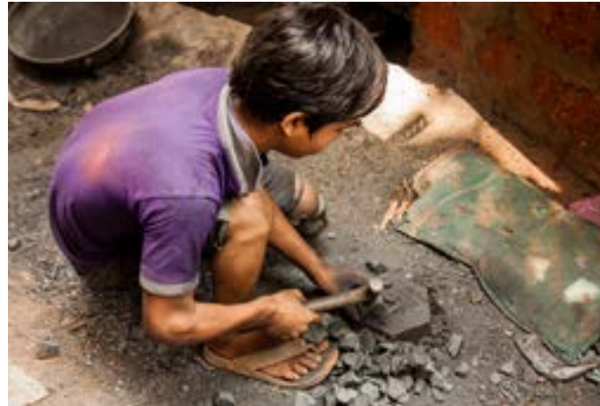
Breaking into a small pieces of stone coal by using a hammer for furnace.
