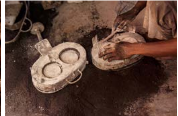
Artisan is carefully taking out the pattern ring after making a pathway.
