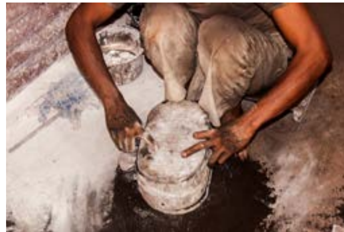
The pattern is taken out and the two box frames are carefully put back together for casting.
