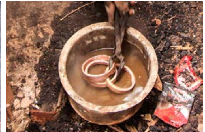
The solidified castings are separated from mold and dropping inside the cold water.
