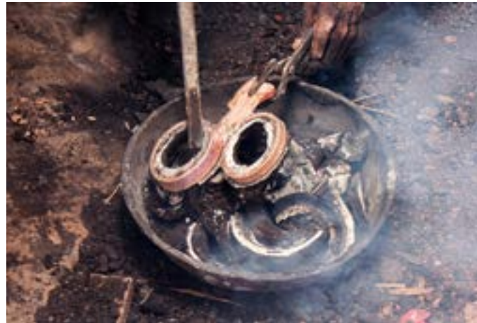
Removing the unwanted mold from solidified casting.
