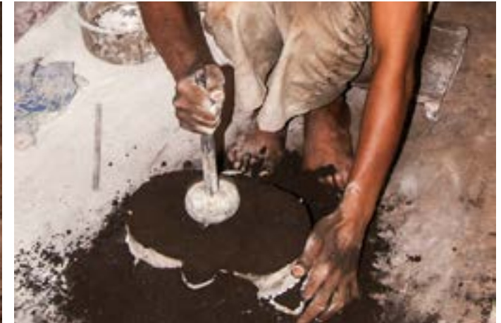
Artisan tightening the soil mixture using round head wooden soil dab.
