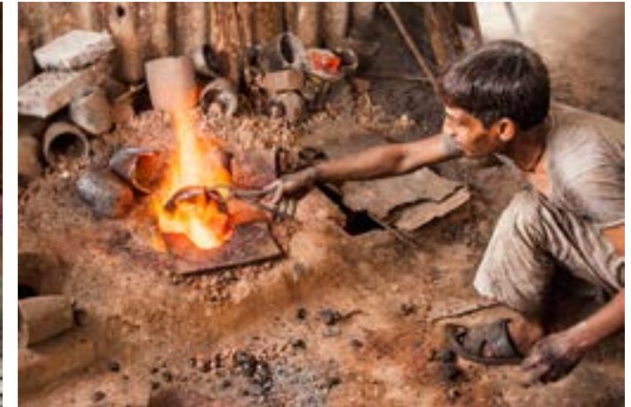
Artisan is heating the old brass metal for its easy to crushing.
