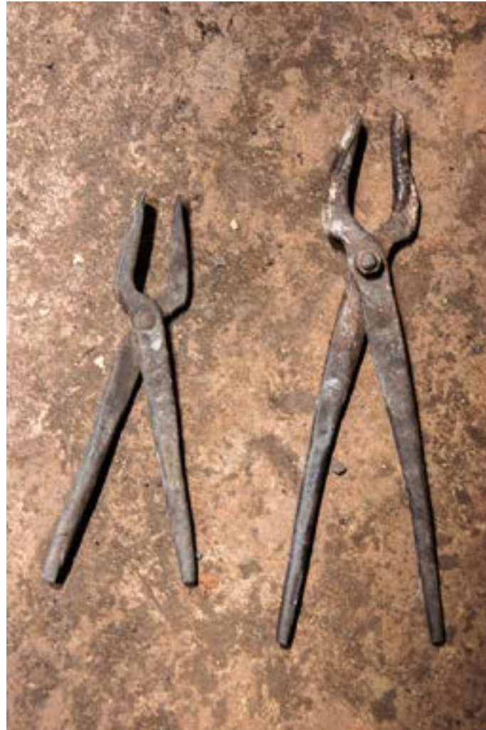
Pincers are used to hold crucibles and other comfortable needs.
