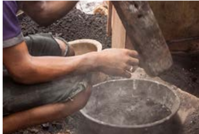
Converting rough soil into soft powder using custom made wooden tool.
