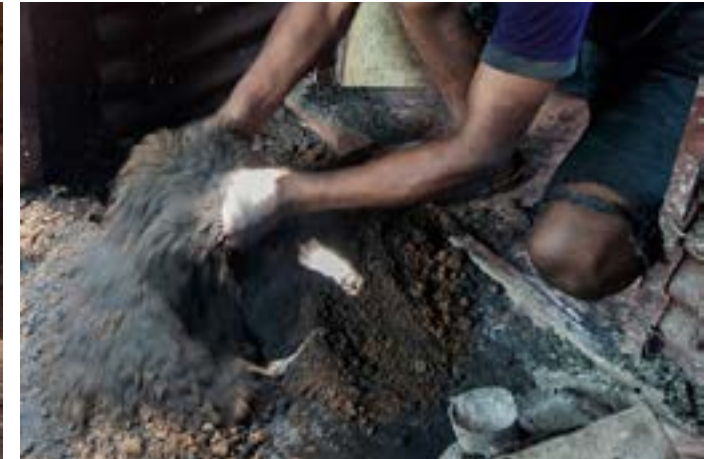
Proper mixing of soil and jungle soil for mold.
