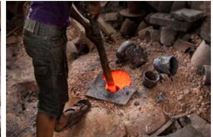
Artist involved in melting old metal in crucible by using custom made furnace.
