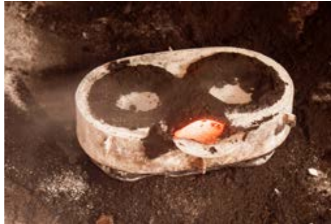
Castings are taken out after cooling the molds.
