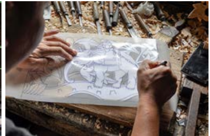
Artisan is sketching on the tracing paper to get printed over the white sheet, which is stuck on the wood.
