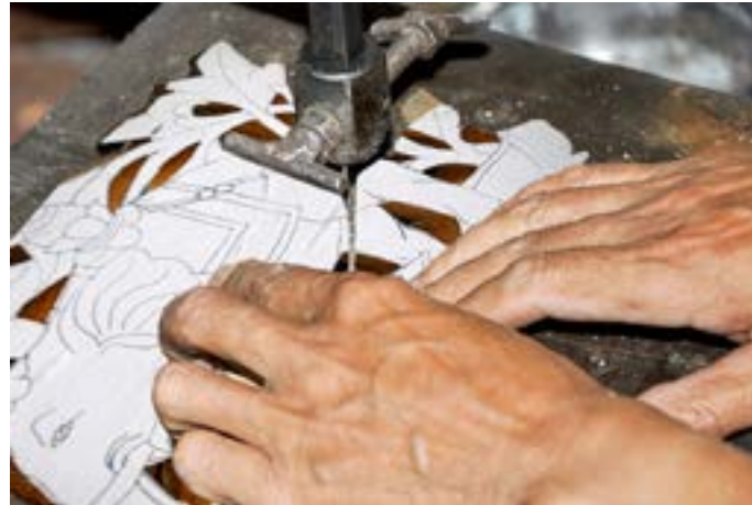
The wood piece is being cut through a band saw as per the designed paper sheet on the wood.
