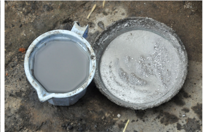
The mixture of copper and zinc powder with water is used to join two parts of the pot.
