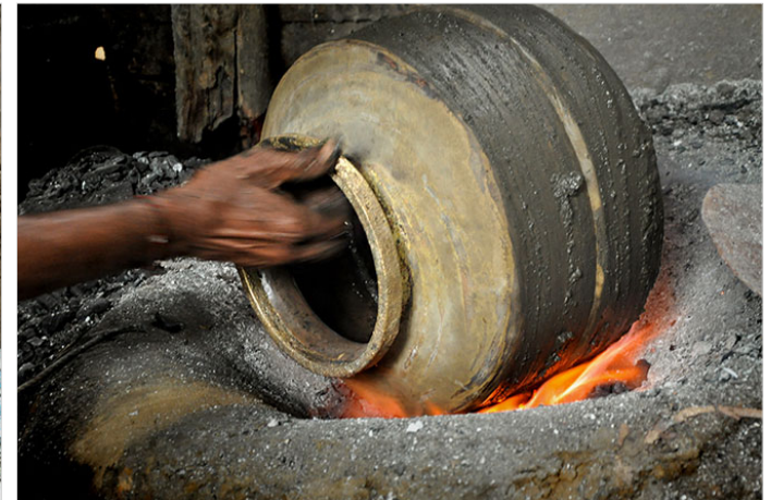
The wet mud applied over the pot is kept for heating.
