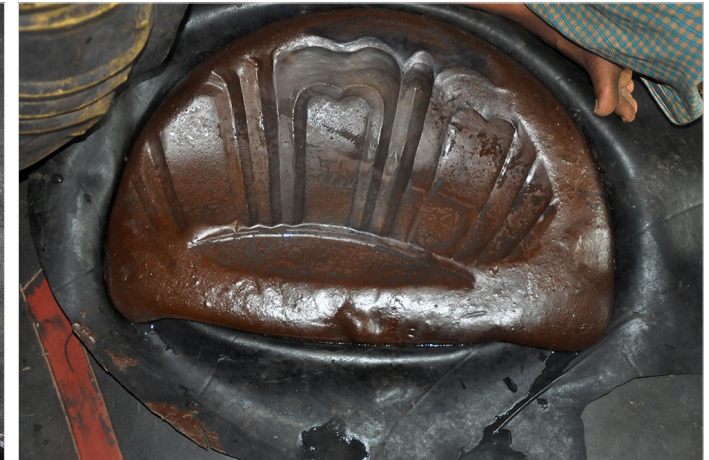
Shellac is used to fill inside the jug to emboss as per the required design.
