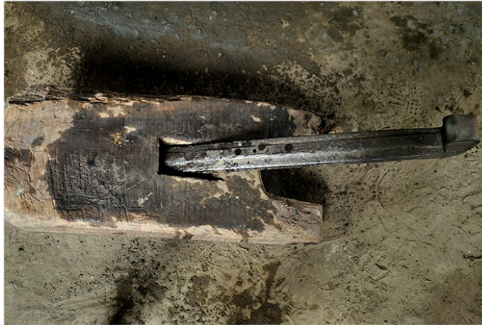
The level tool which is used to shape the pot after heating process.
