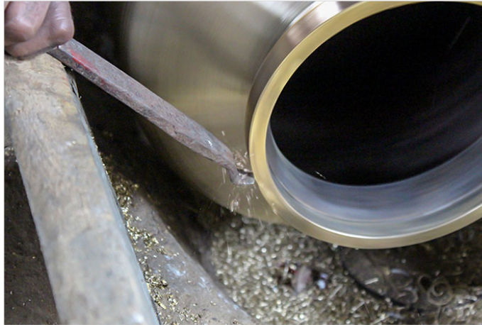
The artisan is scraping out the waste layer over the brass pot.
