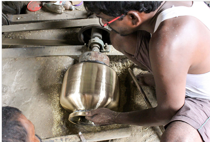
Once the scraping is completed, an artisan is removing the brass pot from the power machine.
