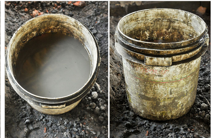
A mixture of mud and water is used to apply over the pot before heating it.
