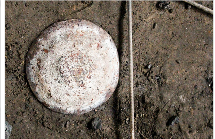
The iron rods are used to rub over the attached part of the pot while heating.
