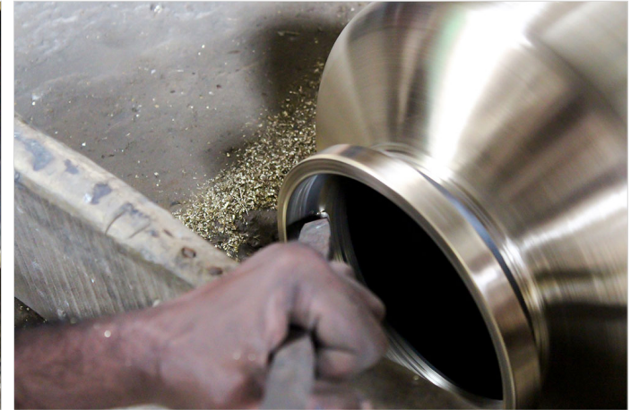
Artisan is scraping the inner layer through the head of the brass pot.
