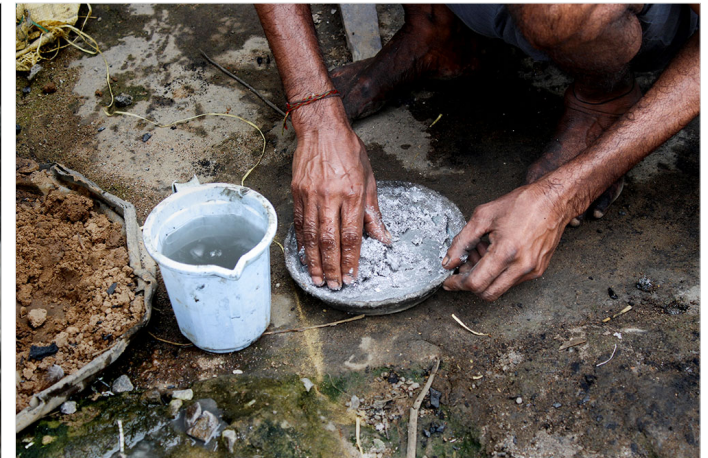
The copper and zinc powder is being mixed with the water to make it into the adhesive paste.
