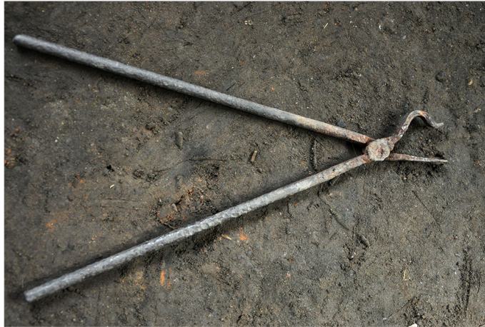
An iron holder is used to change the pot's direction while it is being heated.
