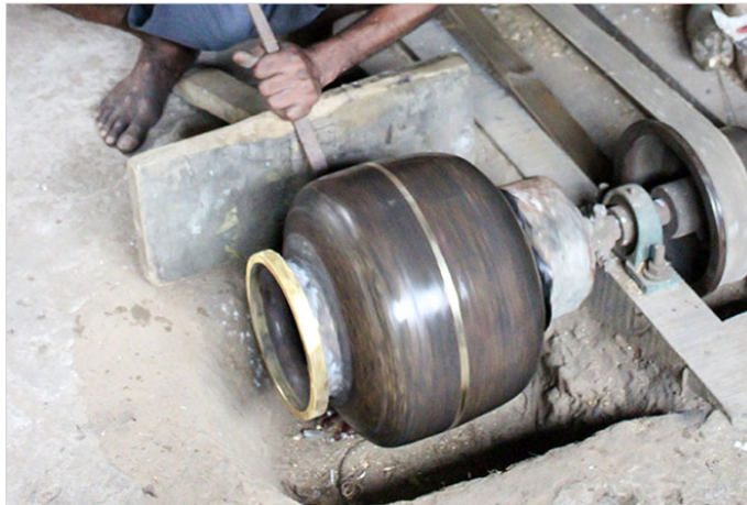
The artisan is placing the sharp iron rod closer to the brass pot and turns on the machine.
