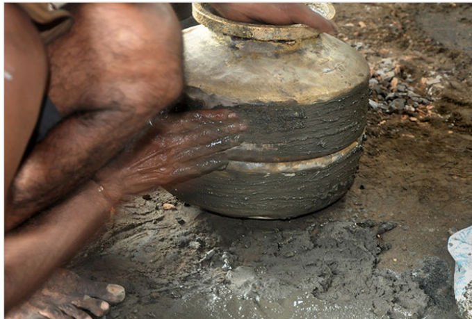
The mixed mud with water is being applied to the pot.
