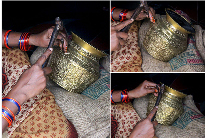
The neck part of the jug is being embossed by the artisan.
