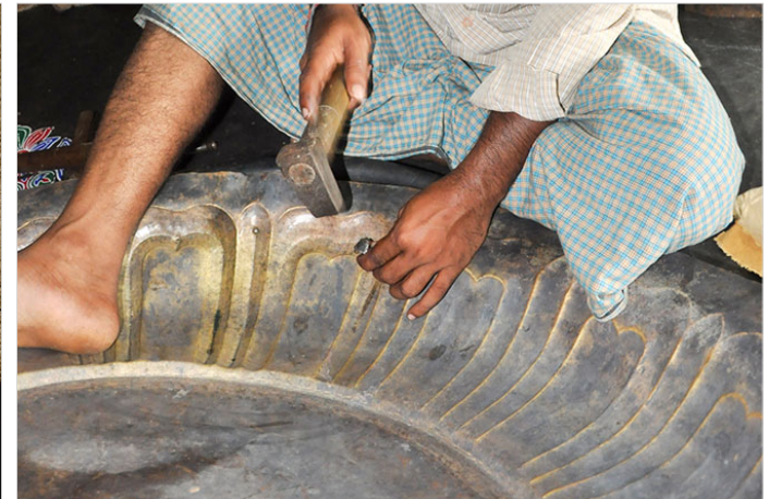
Artisan is embossing the bigger products made up of brass.
