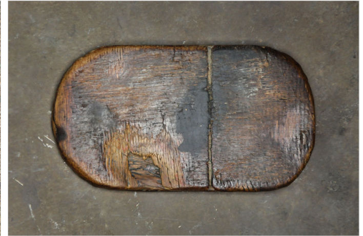
A piece of wood which is used to smoothen the surface of the iron rod.
