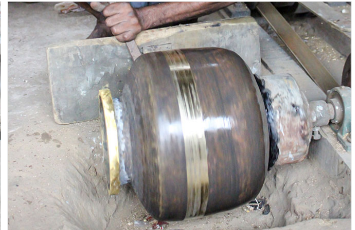
As the machine rotates in high friction, the brass pot is rotating at hyper speed.
