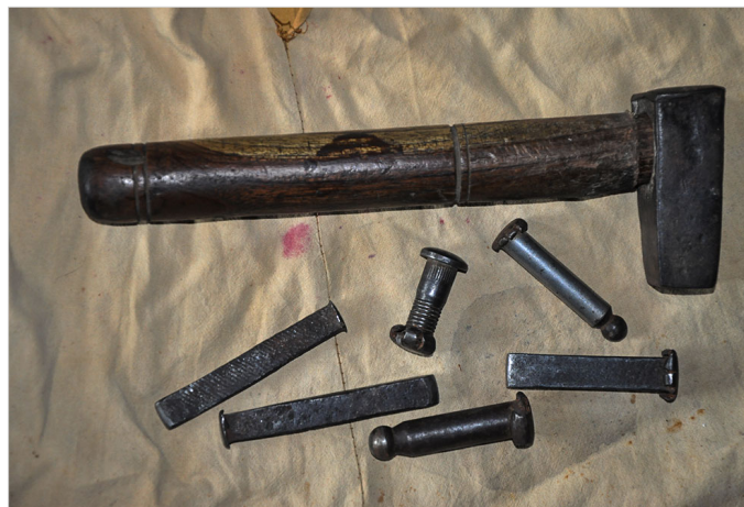
Cross and Straight Pein hammer with small stamping rods to emboss the design.
