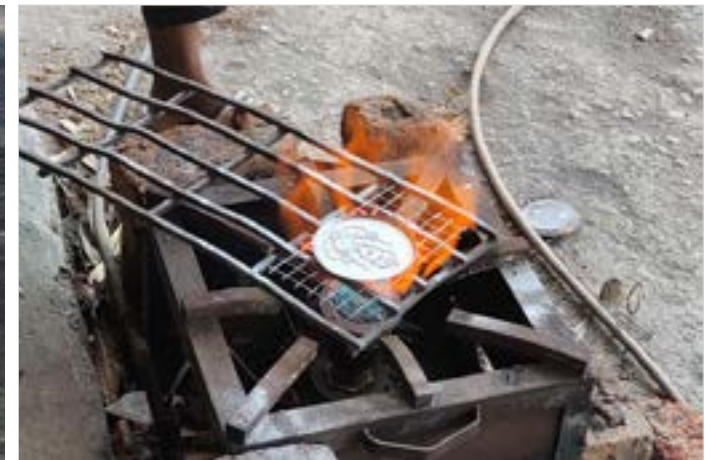
The plate is put on fire for fixing the copper wires.
