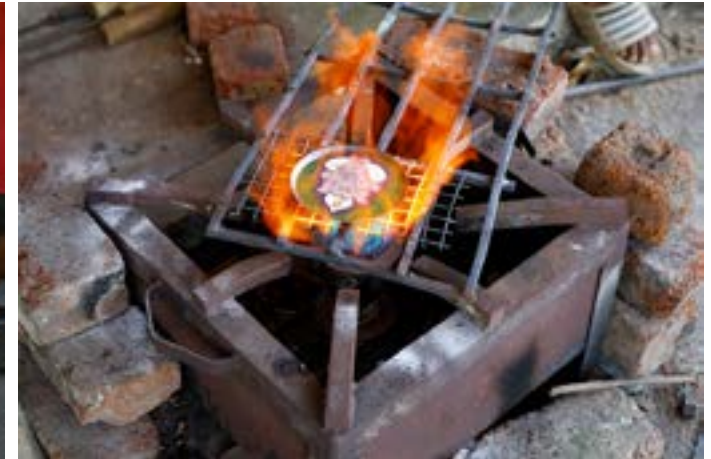
Once again the plate is heated on gas stove to fix the colours.
