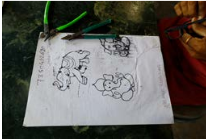
Stencil is used as a reference for cutting copper wire.
