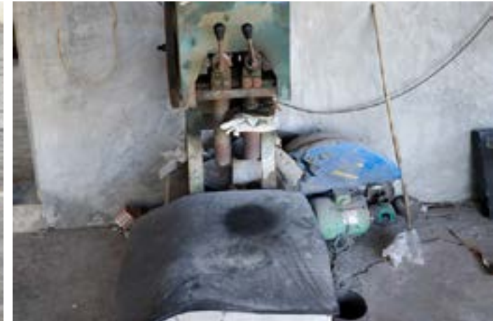
Kandap machine or Pounding machine is used to make colour powder from glass stone.
