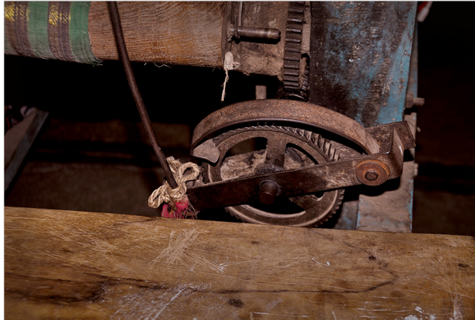
The wheel that helps tighten the weaving machine.
