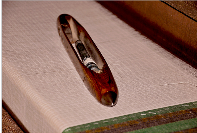
Fly-shuttle loaded with a spindle.
