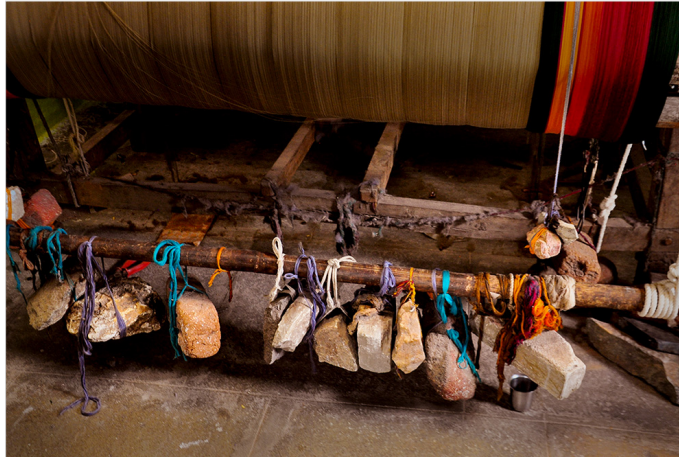
The stone used as a weight to keep a side of the weaving machine tight and intact.
