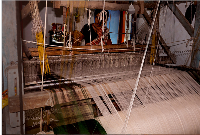
The warp threads being loaded into the loom for the weaving process.
