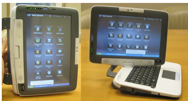
Figure.1 Classmate PC, Intel Learning Series convertible tablet reference design with touch screen
