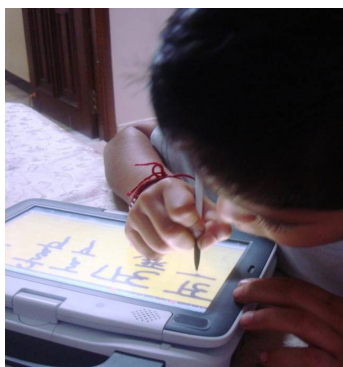
Figure.9 Participant (5 years) writing big alphabets, as the screen is unable to identify detailed pen strokes with varying stylus pressure
