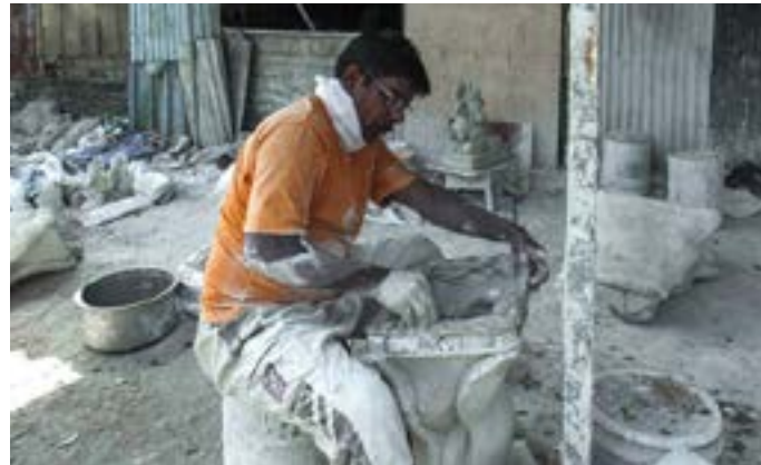
Mold is filled with a paste of PoP.
