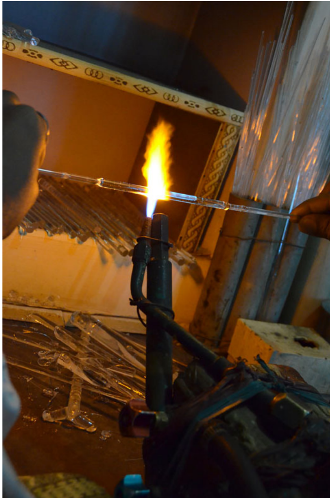
Melting the glass with heat.
