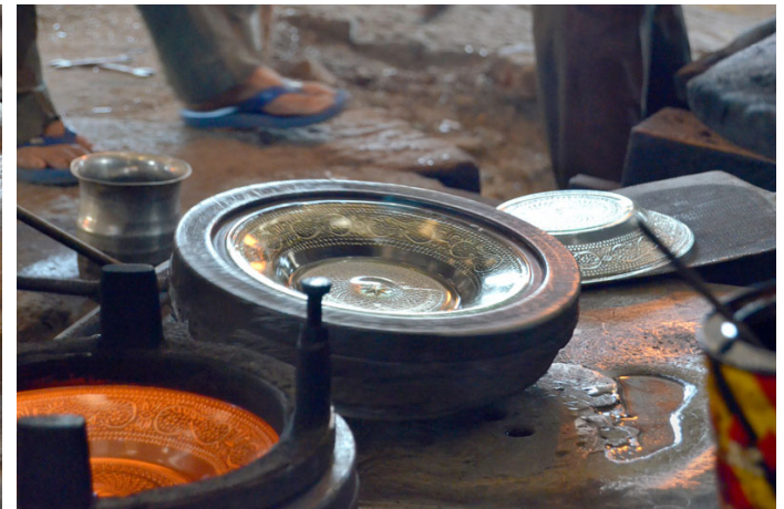
The plate takes the shape of the mould.
