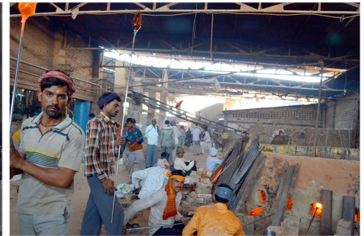
The craftsman getting glass the furnace on a metallic pipe.
