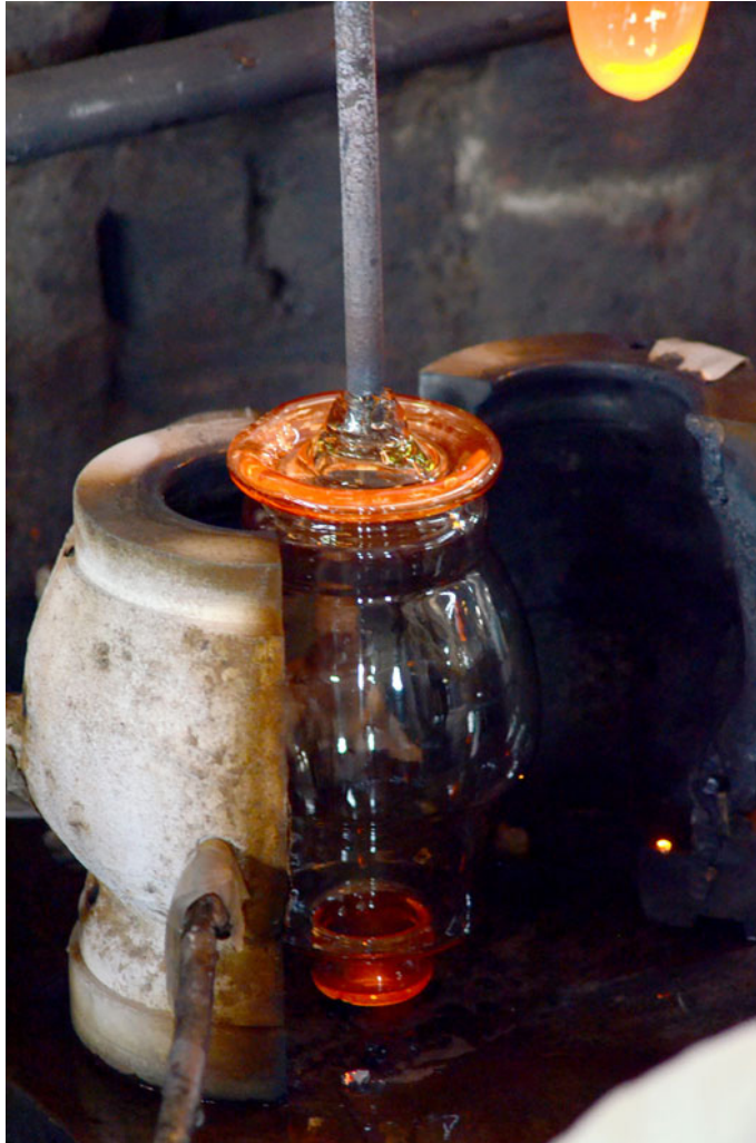
The jar ready to be removed while another gob is introduced in the mould.
