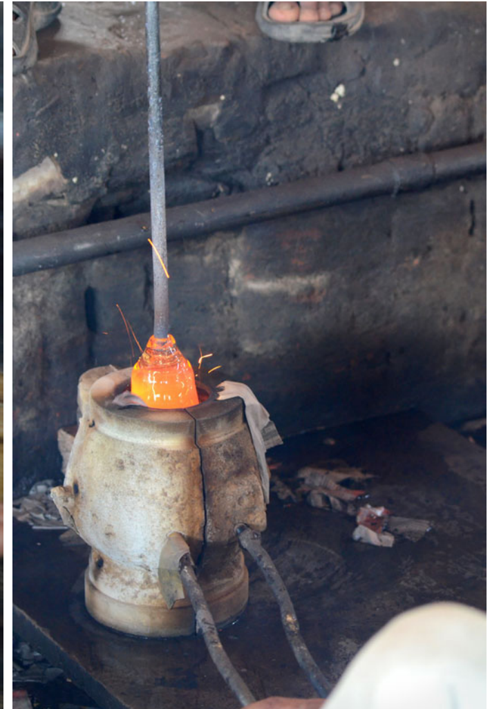
Glass takes the shape of the mould while air is being blown from the other end.
