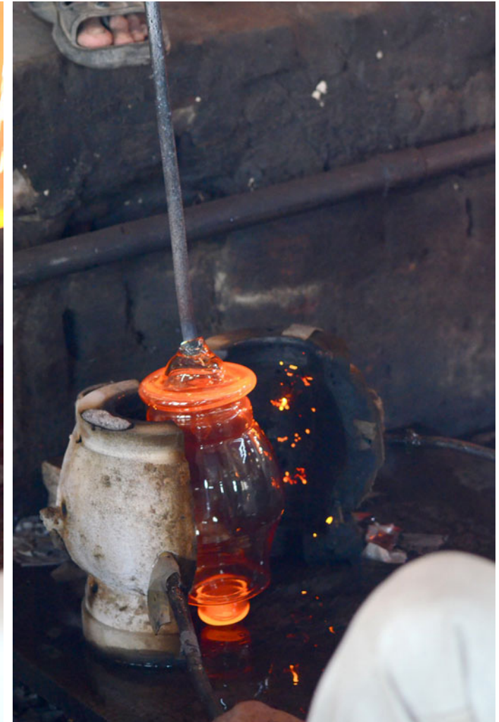
And the jar takes the shape of the mould.
