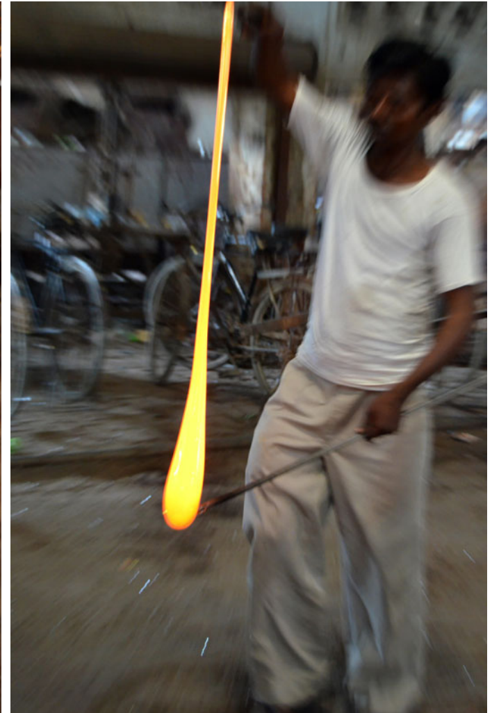
A craftsman preparing the glass stream to be put on to the bangle rod.
