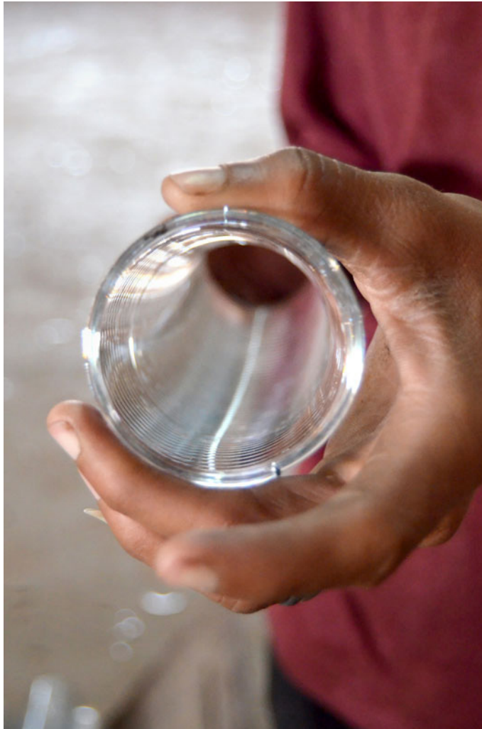
Glass spring generated by coiling the glass.
