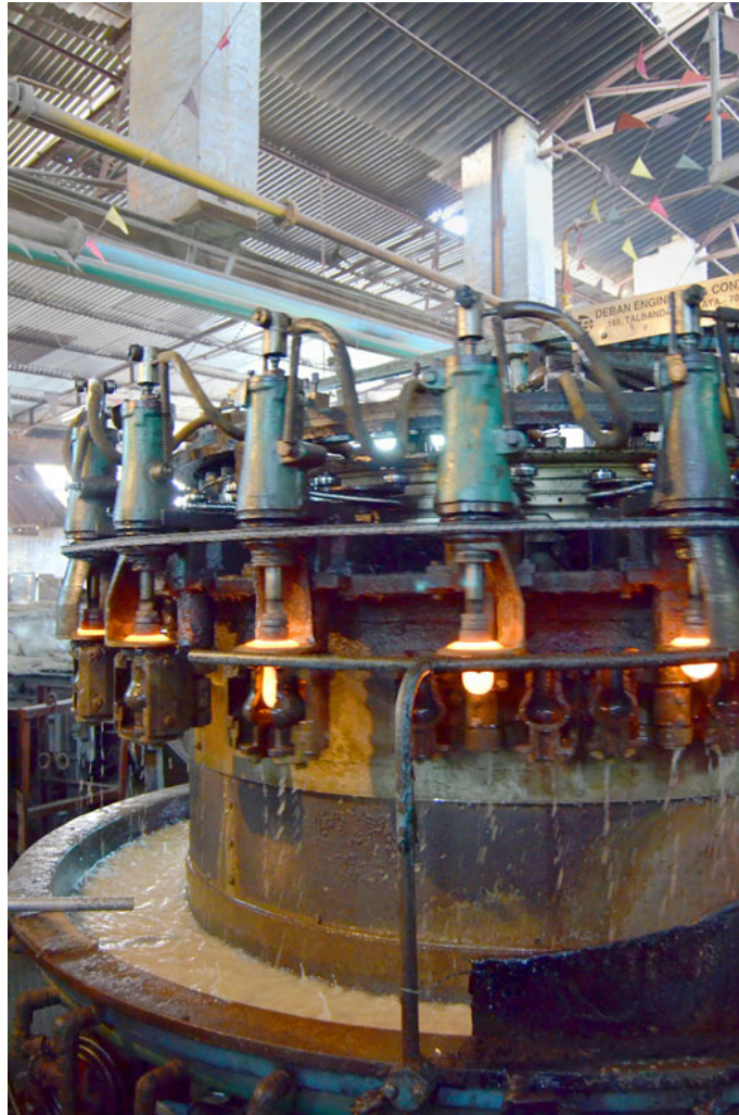
The automatic 'forming machine' making the glass shells.
