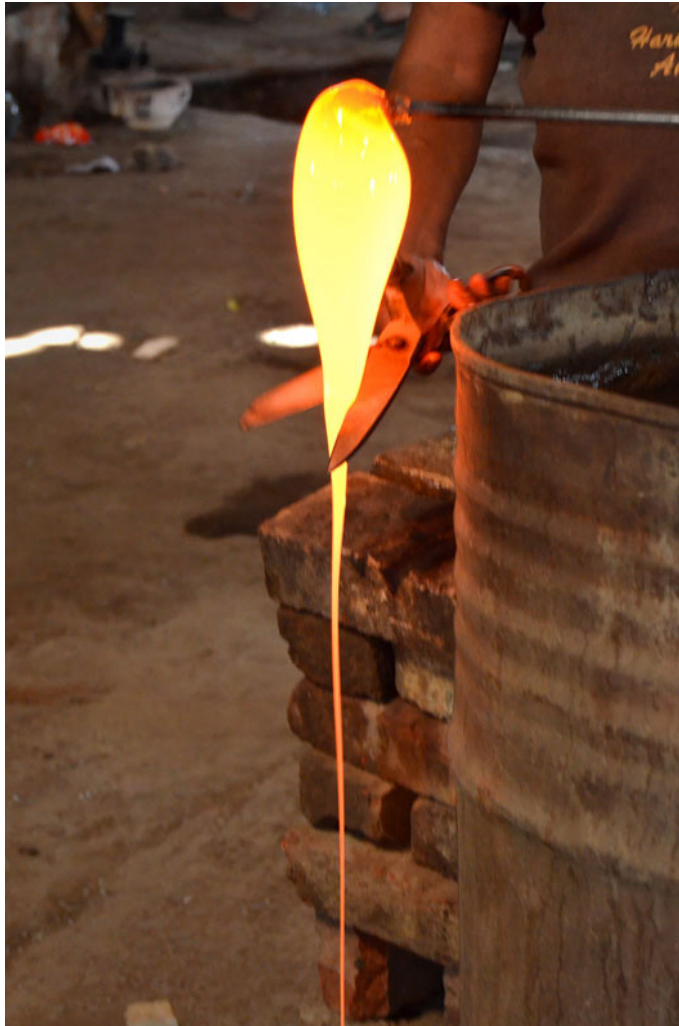
Another glass stream being cut to be coiled into bangles.
