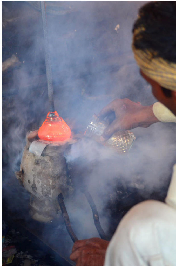
Water being sprinkled to cool off the mould.
