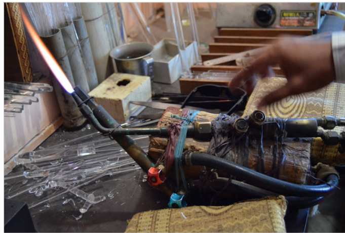
Gas burners for melting and fusing the glass.
