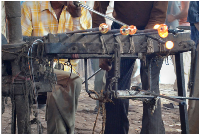
Air being blown from the other end of the hollow pipe.
