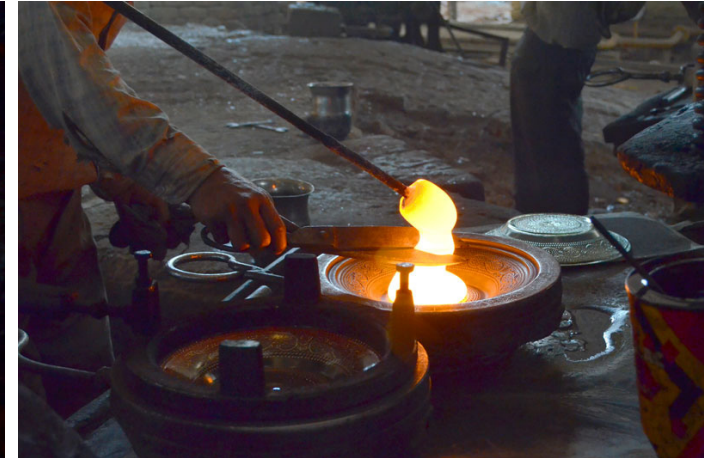
Stream of glass being put in the moulds.
