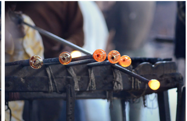
Air being blown from the other end of the hollow pipe.
