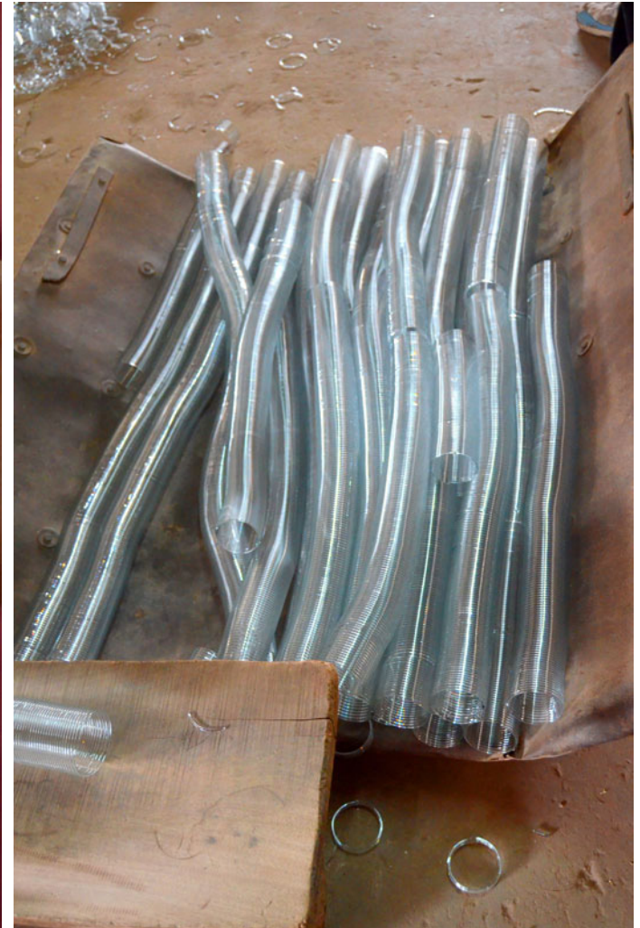
Glass spring generated by coiling the glass.
