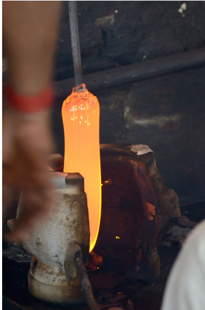
Gob falling by gravity.
