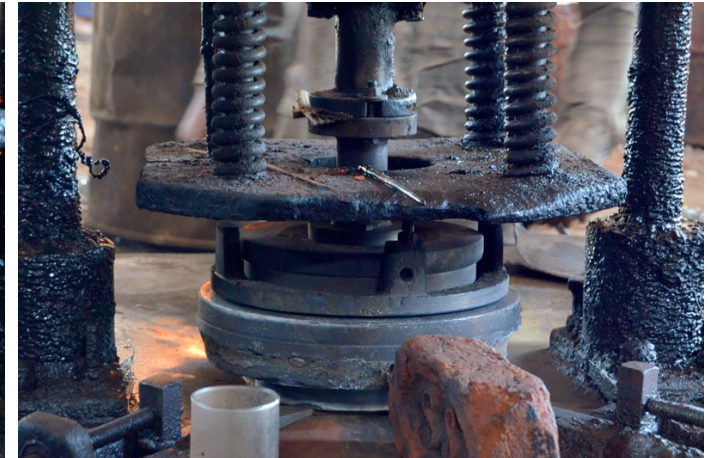
The moulds being pressed against each other to make the plate.
