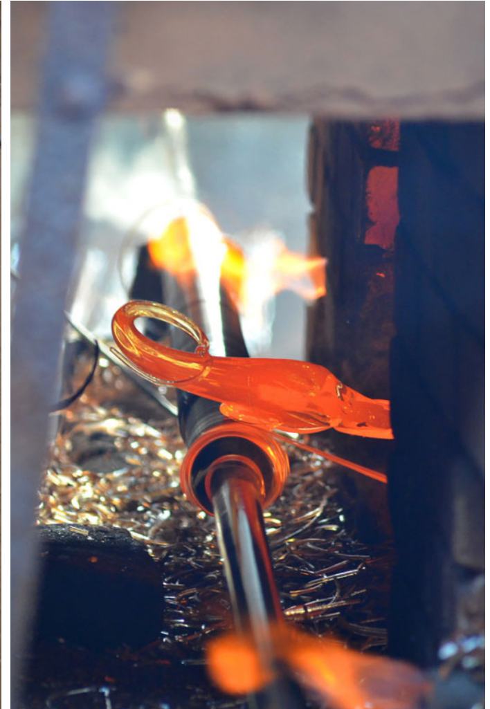
Craftsman putting a thin glass wire onto the bangle-coiling rod.
