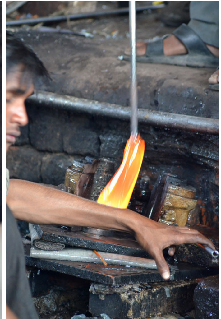
Gob falling by gravity in the mould.
