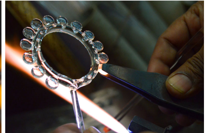
Flattening the circle with a tong.
