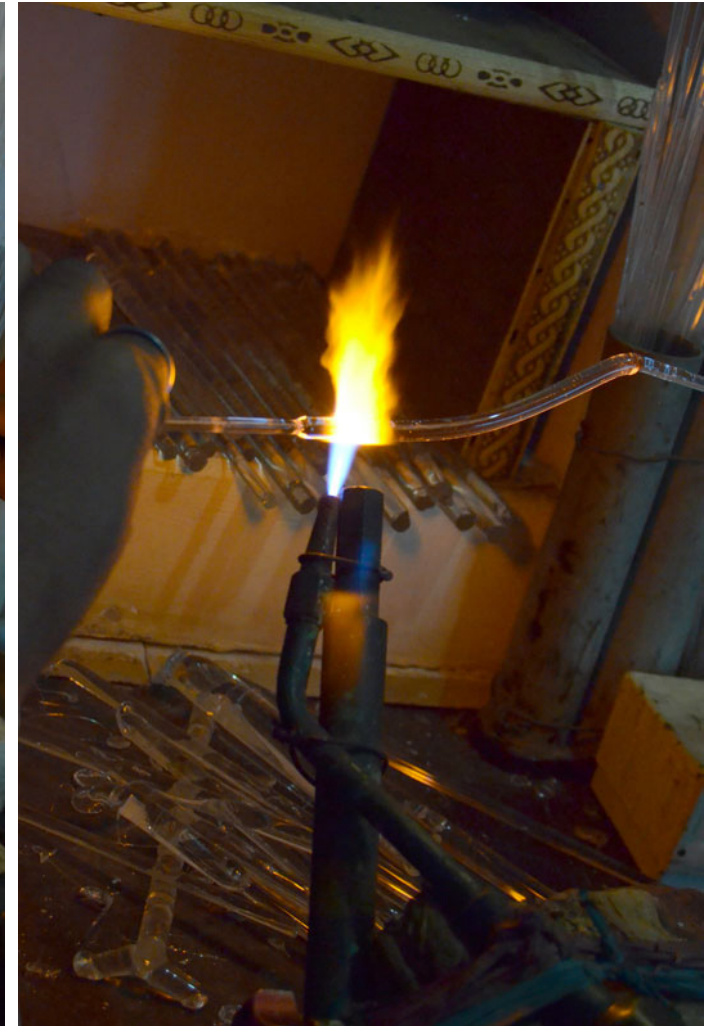
Melting the glass with heat.
