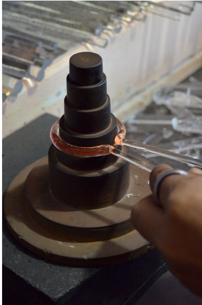
Bangle measuring rings, seen at the bottom is the carbon base that doesn't burn with heat.
