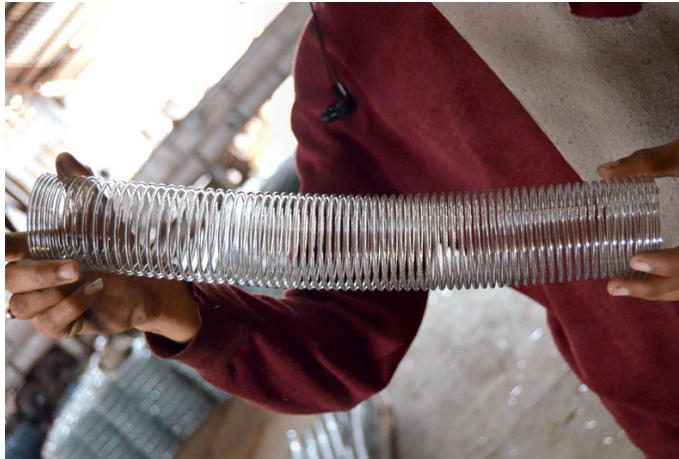
Glass spring generated by coiling the glass.
