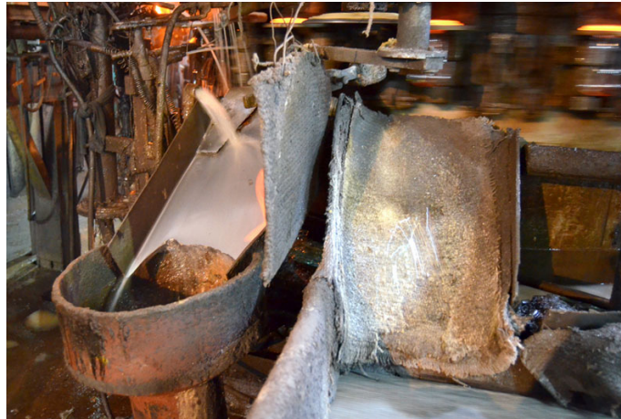
Conveyor belts to cool off the shell.
