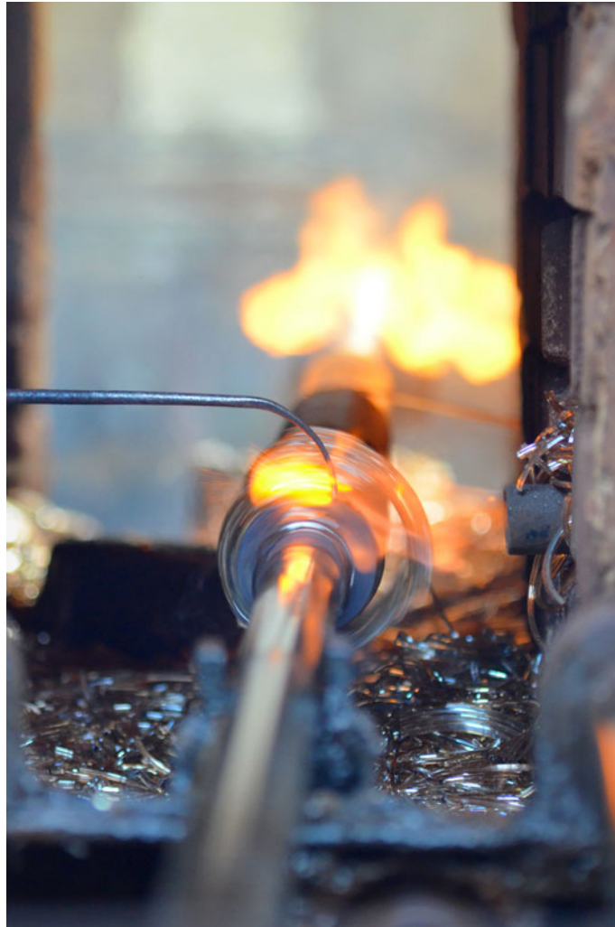
A pointed tool preventing the bangles from sticking with each other.
