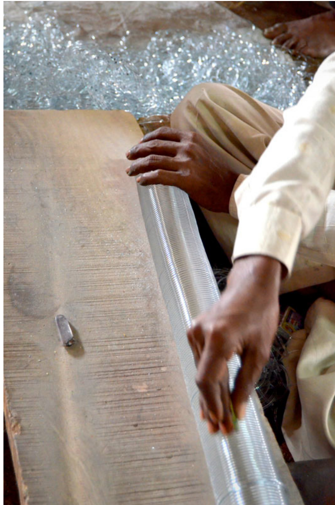
The coil being cut using a diamond cutter, separating the bangles from each other.
