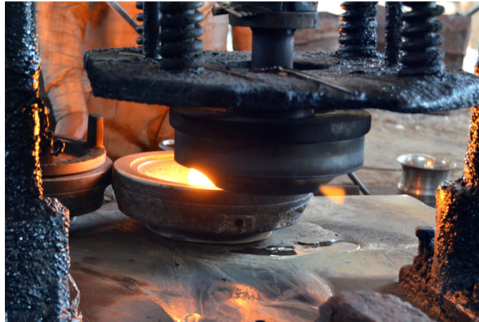
The moulds being pressed against each other to make the plate.
