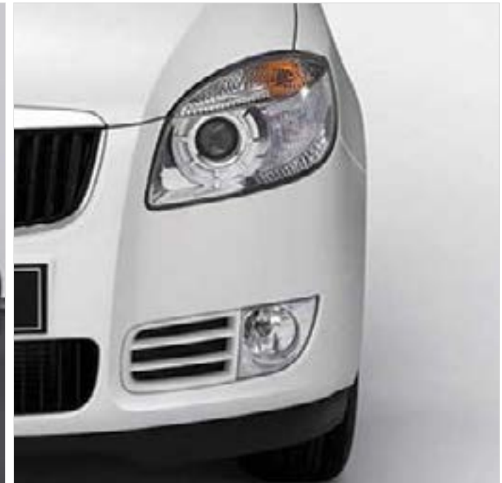
Projector Headlamp in Skoda Fabia (Image source)
