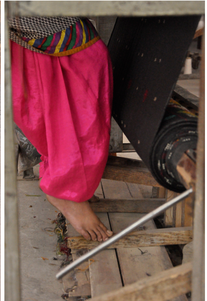
Artisan use pedals to pull the heddle frame up and down.
