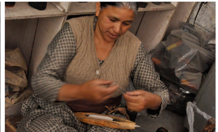
Artisan inserting the spindle to fly-shuttle.
