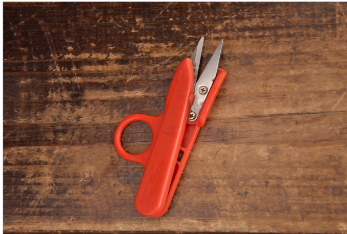
Special kind of scissor is used for cutting the yarn in various processes of weaving.
