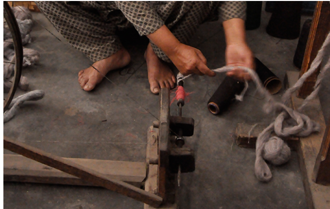
The yarn is extracted from raw wool.
