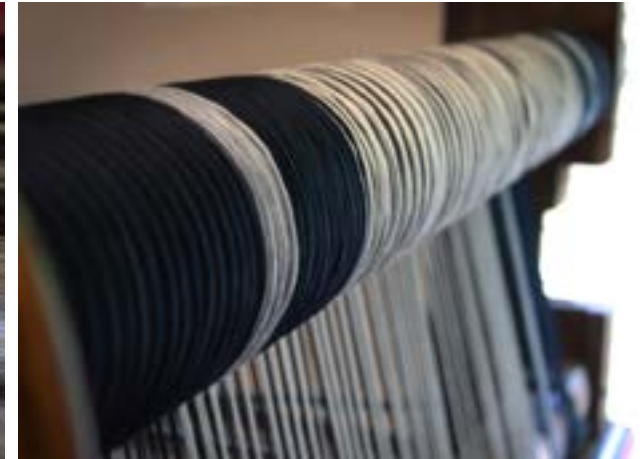
Winded warp beam on the loom.
