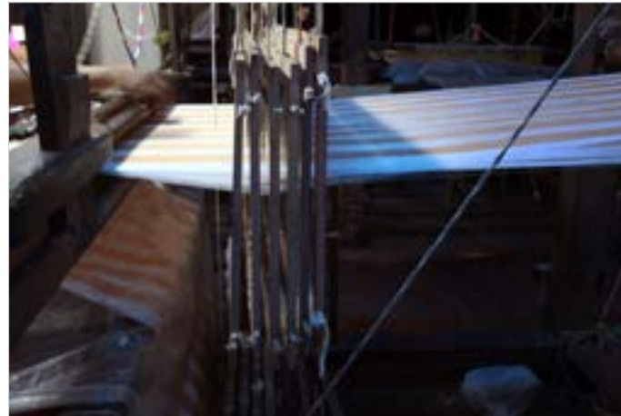
The tiny yarns pass through heddles which gives a definition to the character of fabric.
