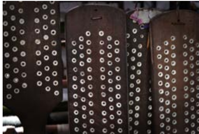
Comb, a specially designed equipment which is used for warping the yarns on warping mill.
