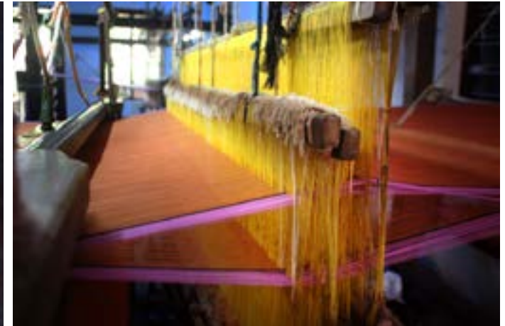
Heddles which plays an impeccable role in the making of fabric.
