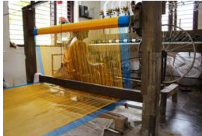
Warp beam of pit loom.
