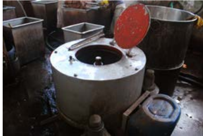
Drying machine which is used for drying yarns after sourcing and bleaching.
