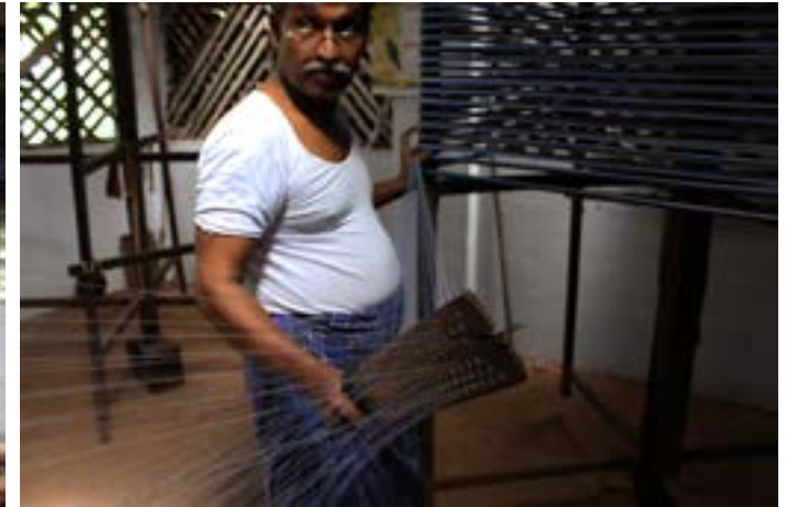
Artisan warping the yarns on warping mill.
