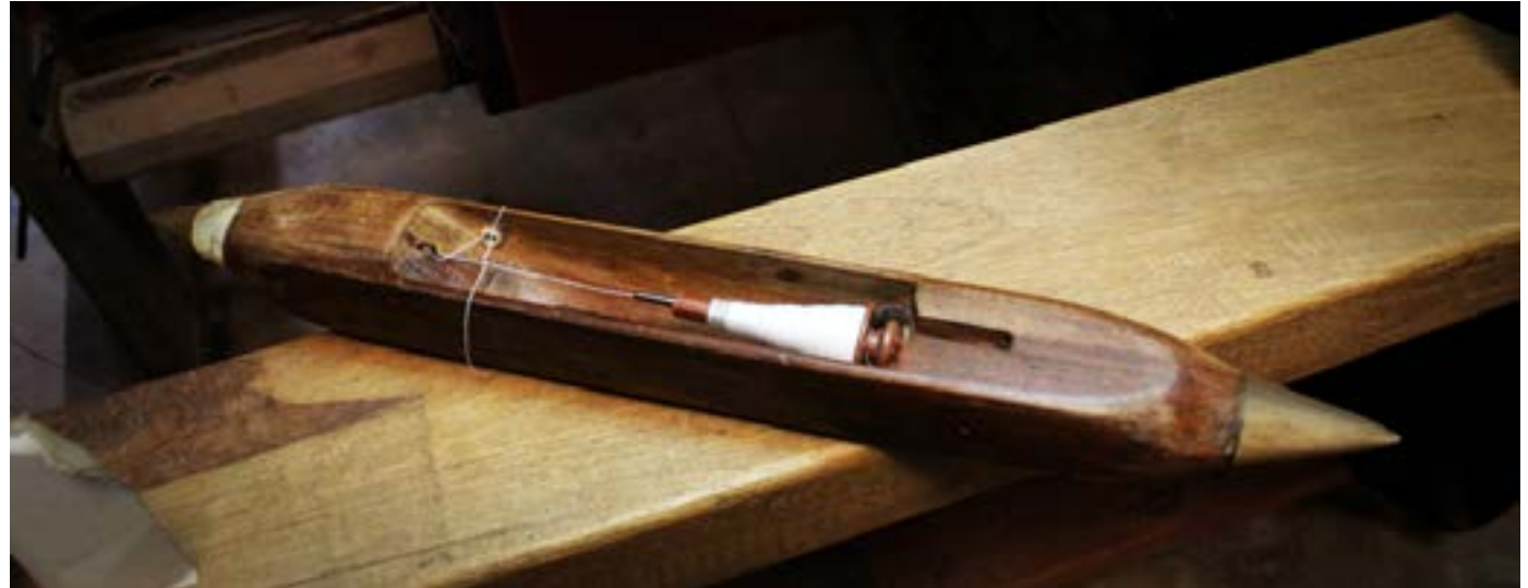
A shuttle is the carrier of weft yarn.
