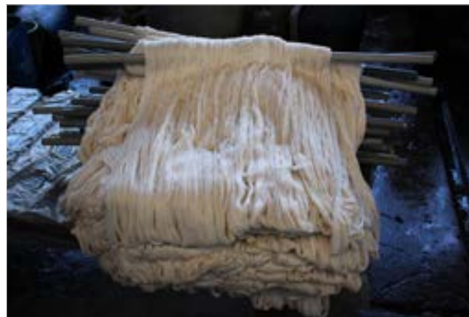
Bleached yarns are kept for draining water.
