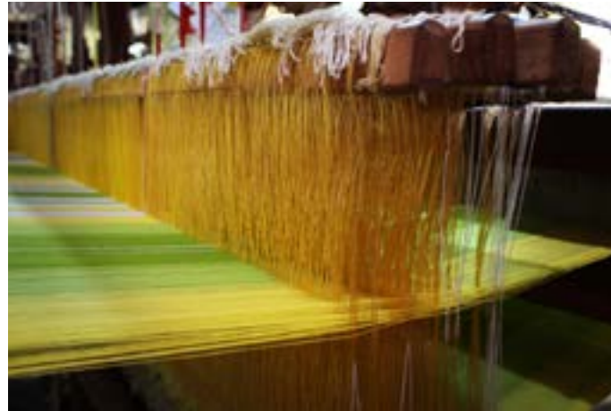
Heddles, the passing way of yarn to fabric.
