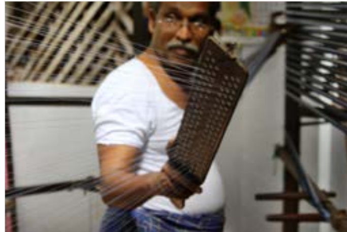
Artisan warping the yarns on warping mill.
