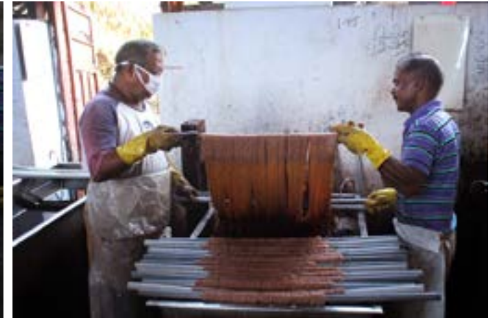
Yarns are dipped continuously in the dye bath to get even coloring.
