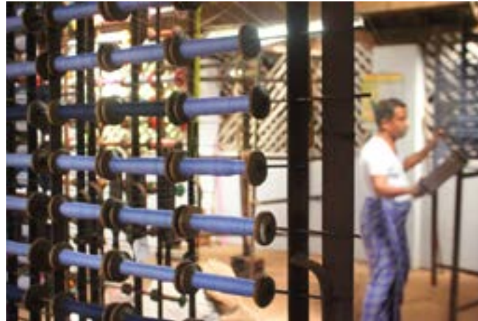
Warping process; a close up view.
