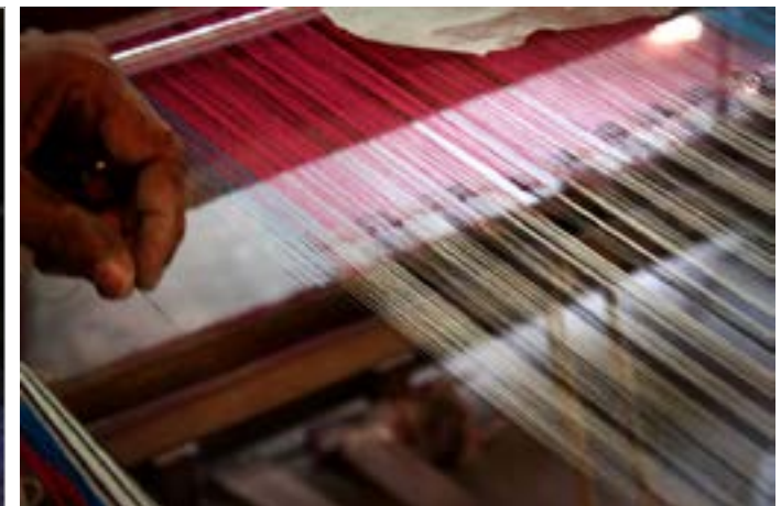
Hands are used to join each yarn to join with the previous yarn during loom setting.
