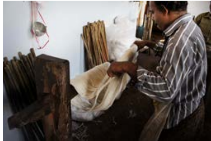
Yarns are beaten on a wooden frame to remove curls and tangles.
