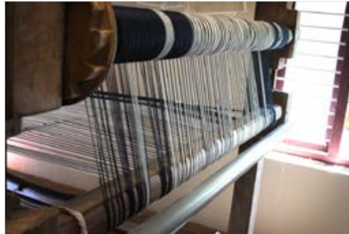
Winded warp beam on the loom.
