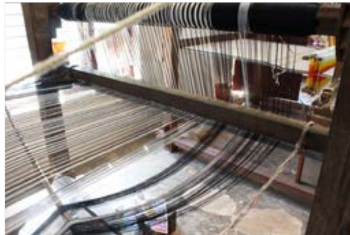
Warp yarns and warp beam.
