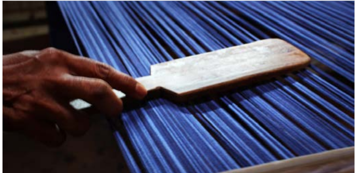
Brushing wax on yarns to avoid yarn breakage.
