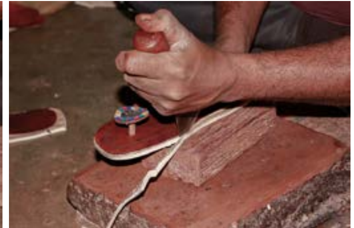
The exceeded parts of the outsole is cut out using chisel.
