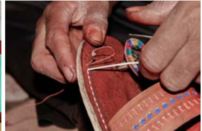
Stitching are made in proper proportion to hold both the sole stronger.
