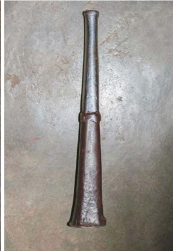
Metal rod is used to press any two parts of sandals during sticking process.
