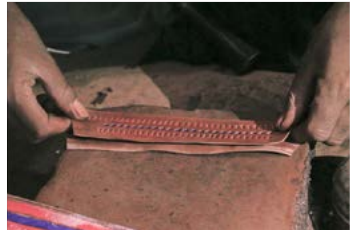
Designed and plain leather is pasted together to give smooth finishing on the bottom of the strap.
