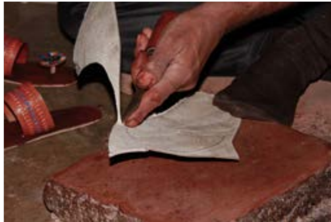
The outsole is cut out into required shape.
