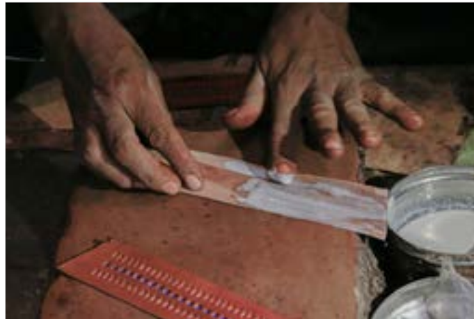
The fevicol is applied on a plain leather to lock the color cloth.
