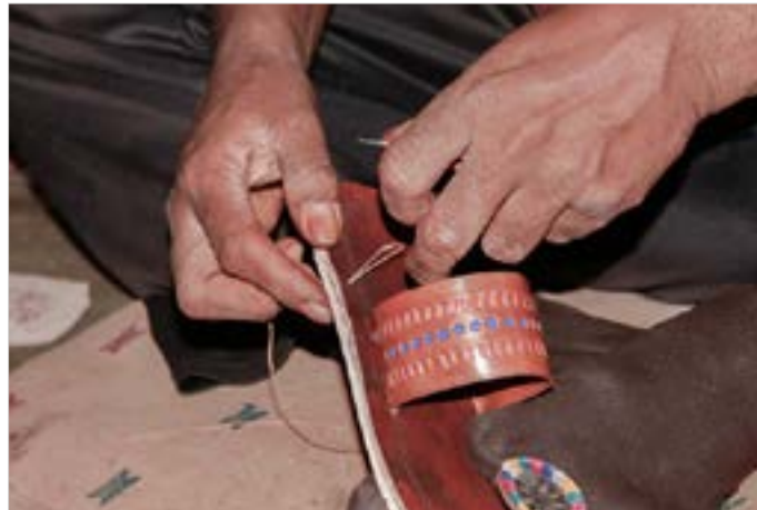
The sandal is stitched to hold both parts tightly.
