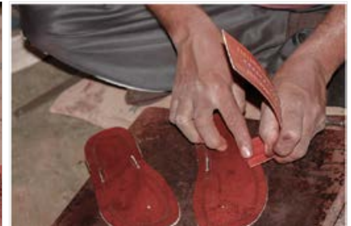
Straps are placed inside the hole.
