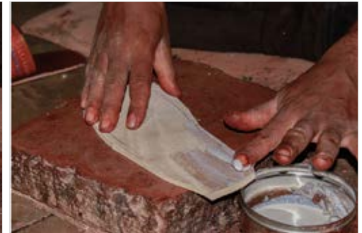
Fevicol is applied on both insole and outsole of the sandal.
