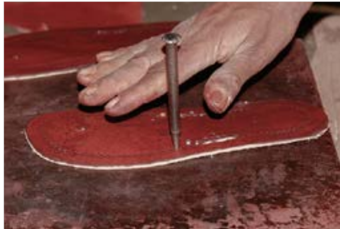
Holes are made on the insole to place the straps in it.
