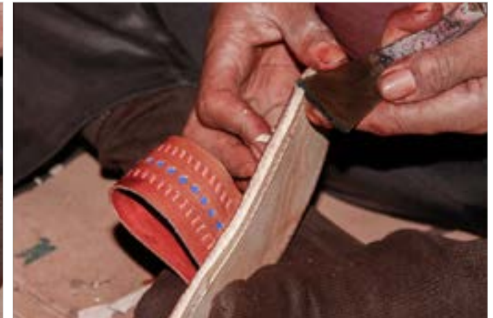
Final shapening of the sandals is done using chisel.
