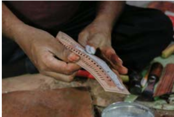
Fevicol is applied on back side of the leather strap.
