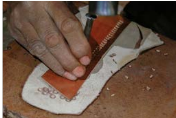
The designs are made by punching the leather using chisel and hammer.
