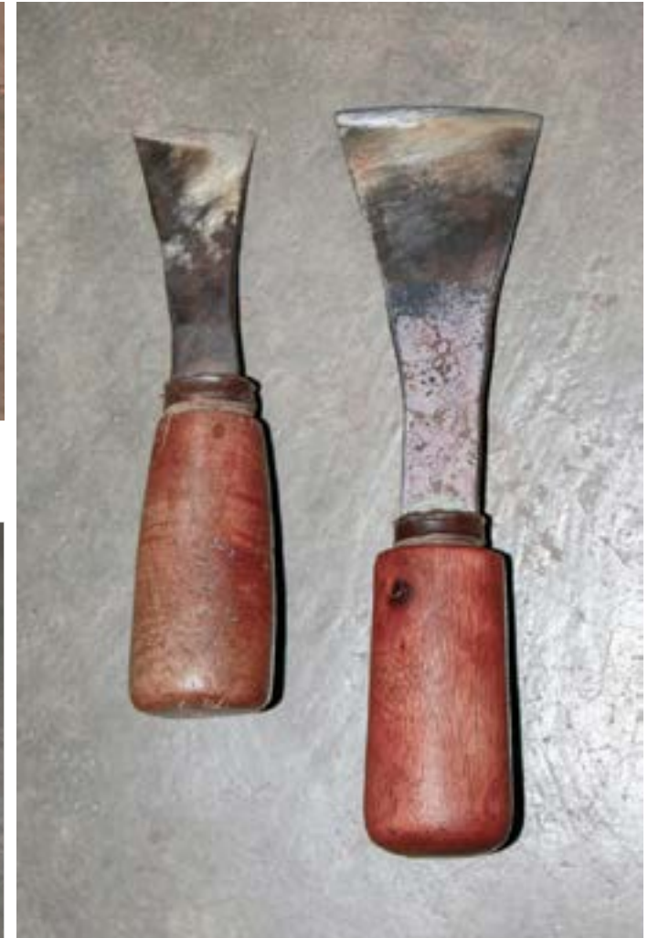
Different sizes of chisels are used to cut the leather and to shape the sandals.
