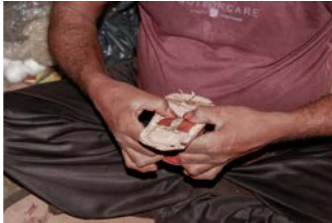
The straps are locked on the back of the sandal using fevicol.
