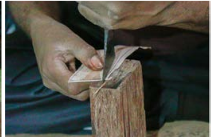
The leather is cut out according to the required size.
