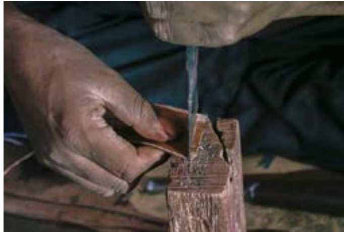
The exceeded part of leather is cut out using chisel.
