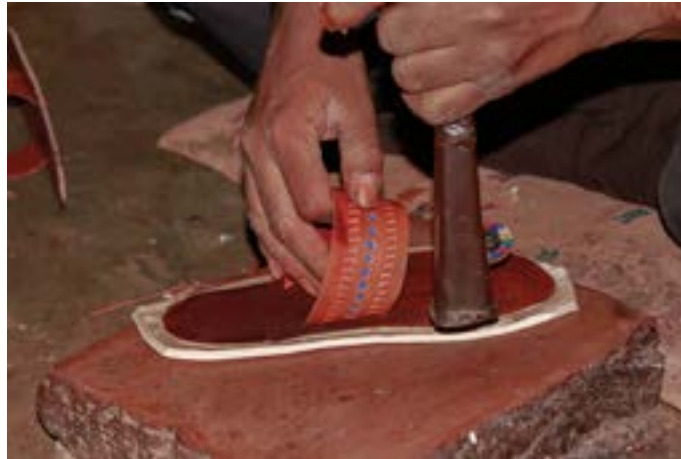
Both the parts are placed together and pressed with iron rod to stick tightly.
