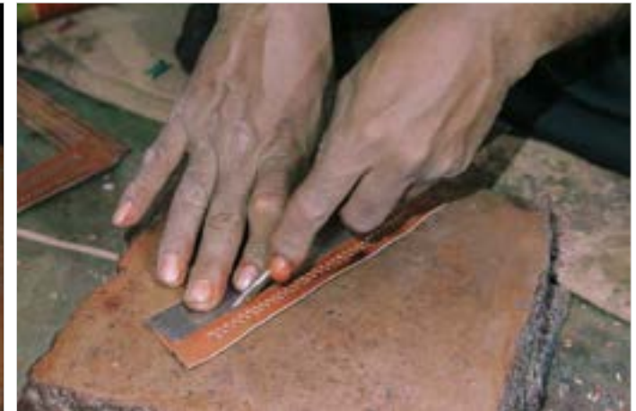
A line is marked as design using screw driver.
