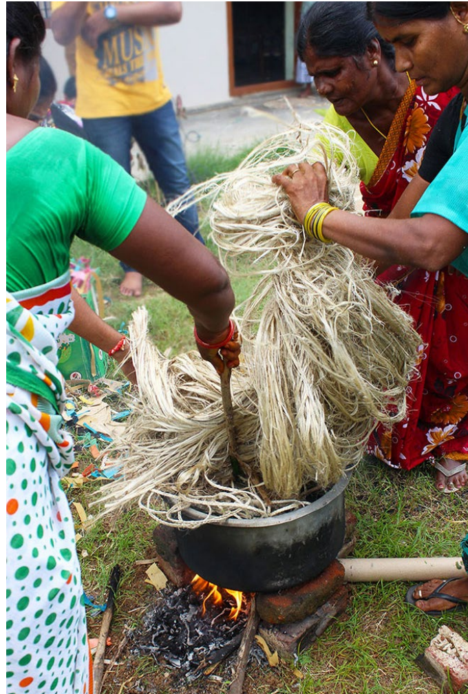
Artisans submerge the jute fibers into coloured hot water.
