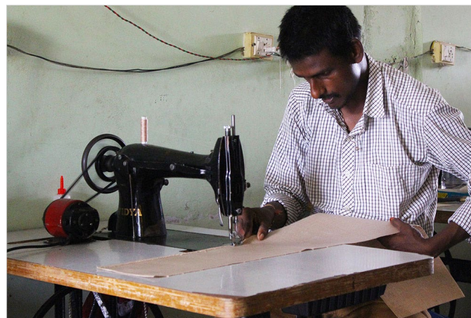
With the help of sewing machine, artisan stitches picot stitch (a loop of thread created for functional purposes along the edge of lace or fabric) at the ends of the fabric to avoid it from fraying.
