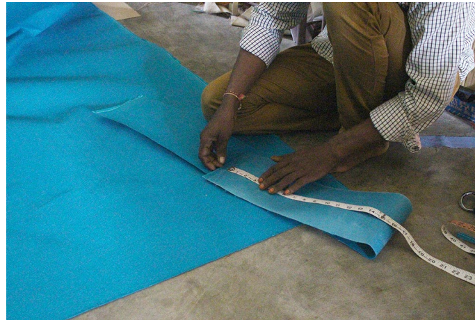
Artisan measures the jute fabric using a measuring tape.
