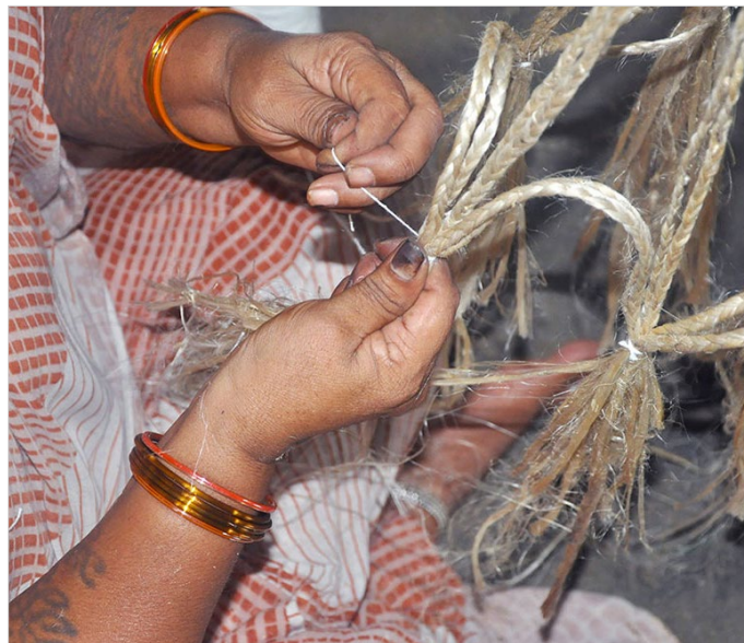
Artisan combines six braids of jute by tying them together with the help of thread.
