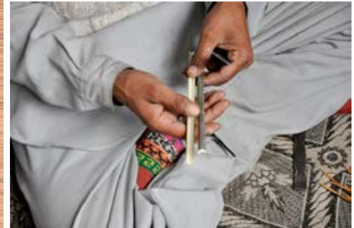
Similarly, bamboo of equal length is split into two.
