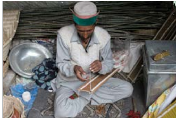
Split canes are tied at the end of bamboo ribs to not to come out.
