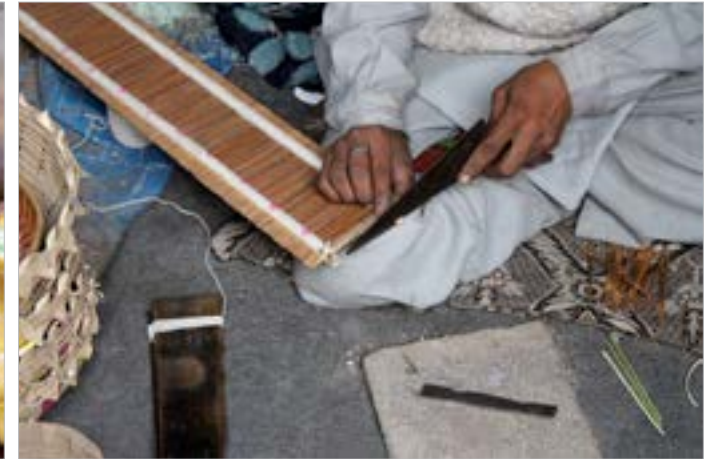
Finishing the work by cutting the end of the split bamboo.
