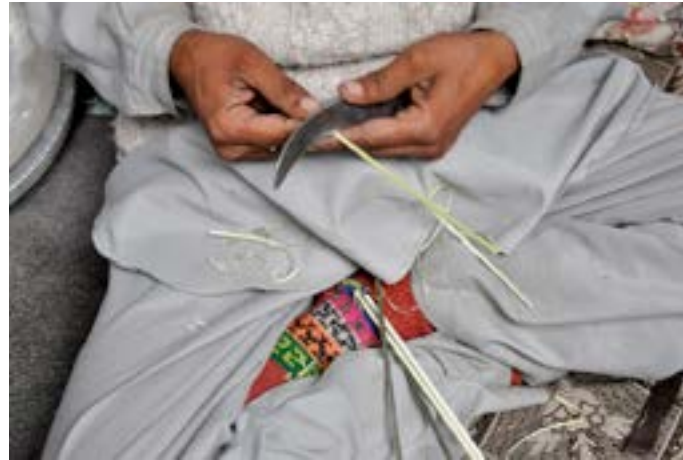
The strips are shaved to the required size by using a sickle.
