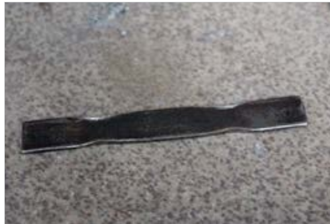
A metal strip is used to tap on the ribs to reduce the space between them.
