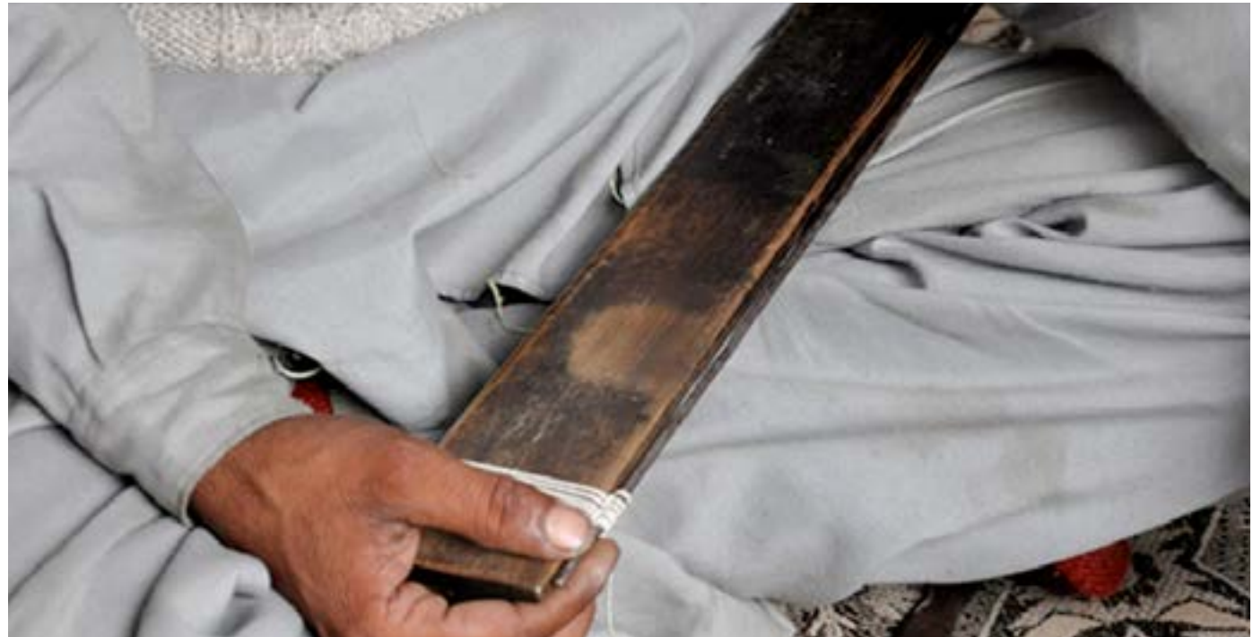
Every dent is measured using the template and it is cut to the required size.
