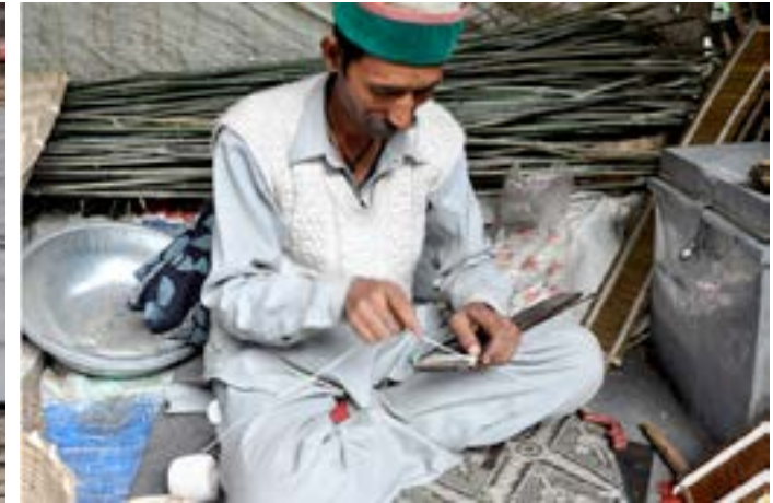
The artisan has a template for the exact length of the dent.
