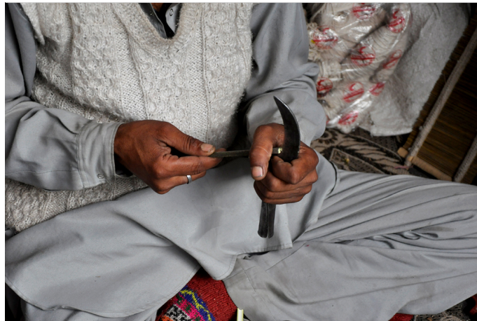
The bamboo is split exactly in the center using a sickle.
