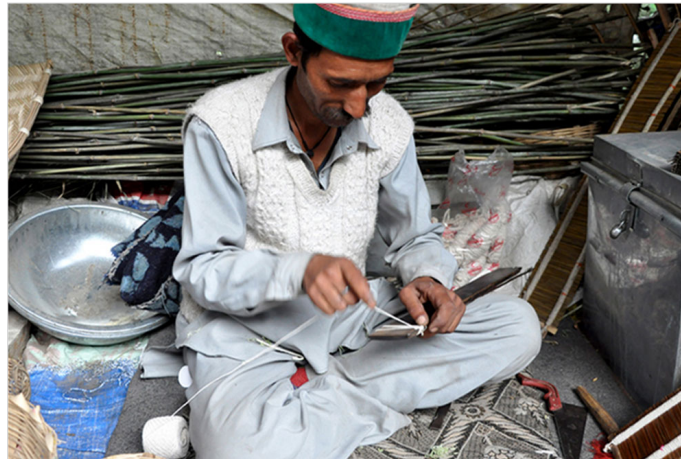
The artisan has a template for the exact length of the dent.
