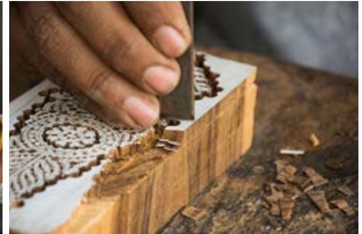
Chipping Motion: Chipping away with the sharp edge of the Farsi.
