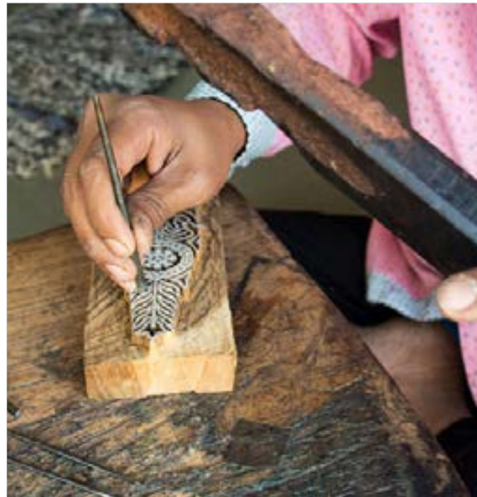
Chetanbhai carving out the edges of the designs, a process that the craftsmen also refer to as 'Safai' which means cleaning up.
