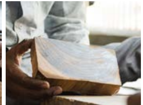
A leveled and polished block ready for the next step in the process, that is, etching.
