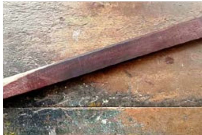
A heavy Thapri used for beating down wood and chiseling.
