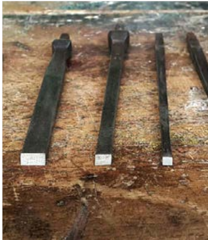
Farsis used for the chipping of excess wood.
