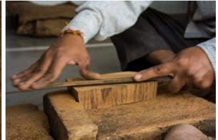
Leveling the block with a hand file on a wooden slab designed to hold the block in place.
