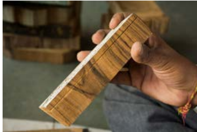
Making such a groove allows the edge to chip off.
