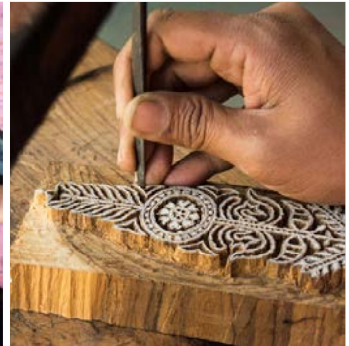
The inner edge of a curve being cleaned with a Gol Punthia or rounded Takna.
