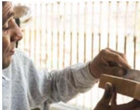
Artisans must check the uniformity of the surface after every round of filing and leveling, done usually with a thick steel scale.
