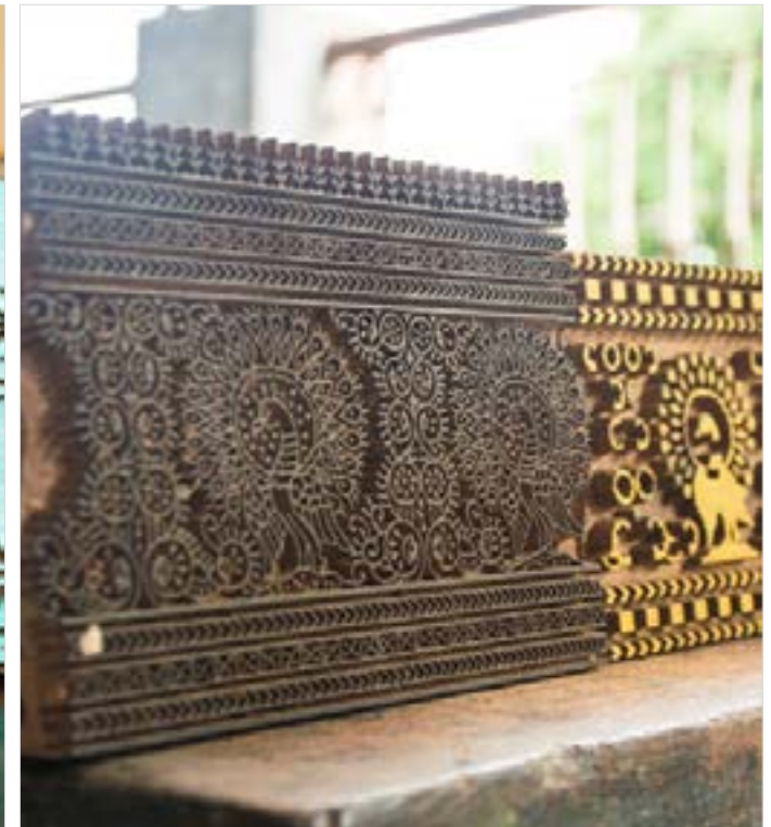
A Rekh (outline) and its corresponding Dattla (filler) block.
