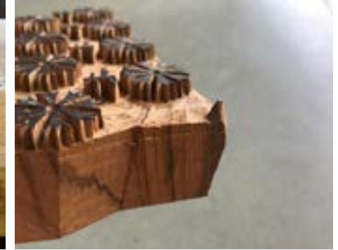
The projection on the corner is a repeat point made with a blunted nail with the wood around it carved in order to support it
