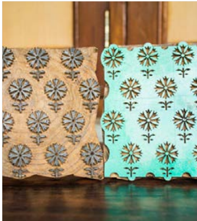
A Rekh (outline) and its corresponding Gad (background) block.
