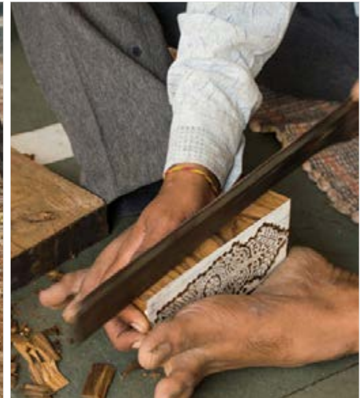
Marking the depth of the block with a saw, an important step.
