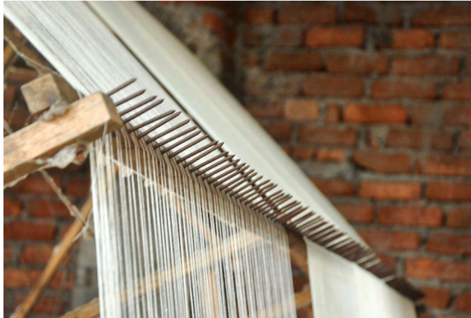
Nails help to avoid misalignments of threads on the warping machine.
