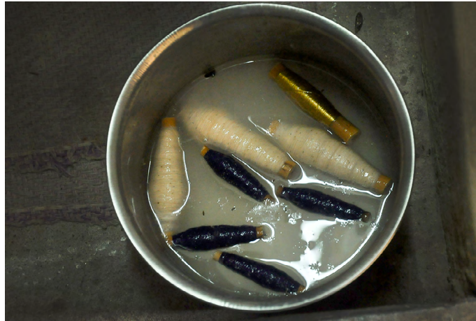
Pirns soaked in starch water.
