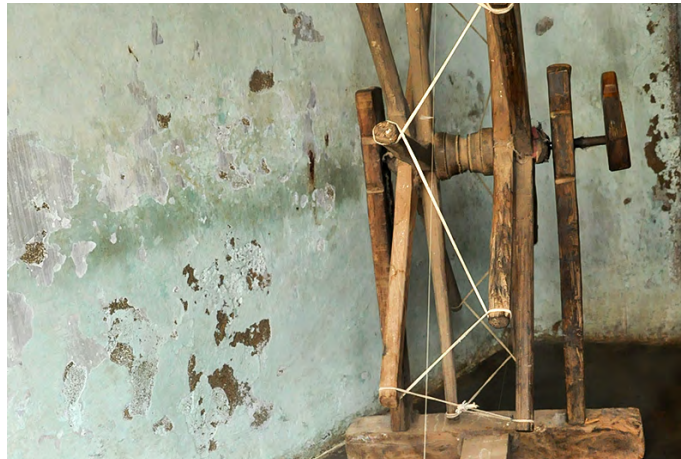
Thread Spinning Wheel is used to obtain thread from cotton fluff.
