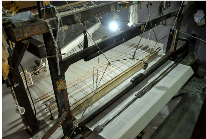
Warped yarns are loaded into the loom for the weaving process.
