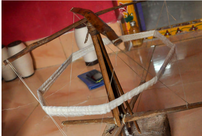
A customized tool is used to segregate yarns in sequential rows.
