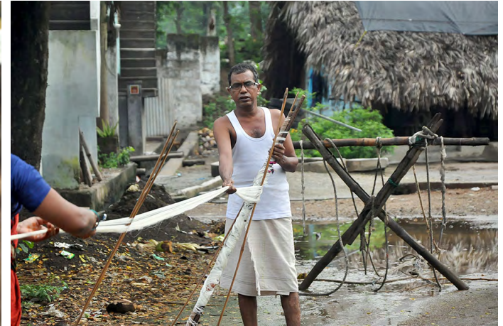
According to the length decided by the artisan, bamboo sticks are repeatedly added at a certain distance.
