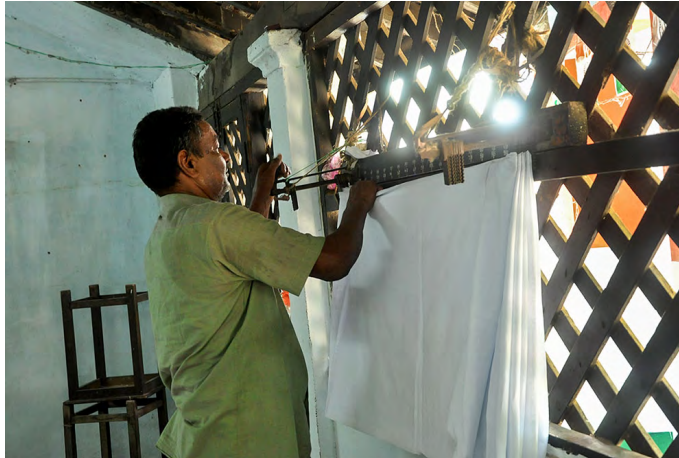
Weaved fabrics are measured using a cloth measuring meter.
