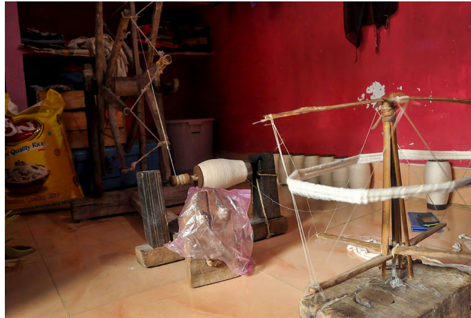
Yarns are attached to a charkha.
