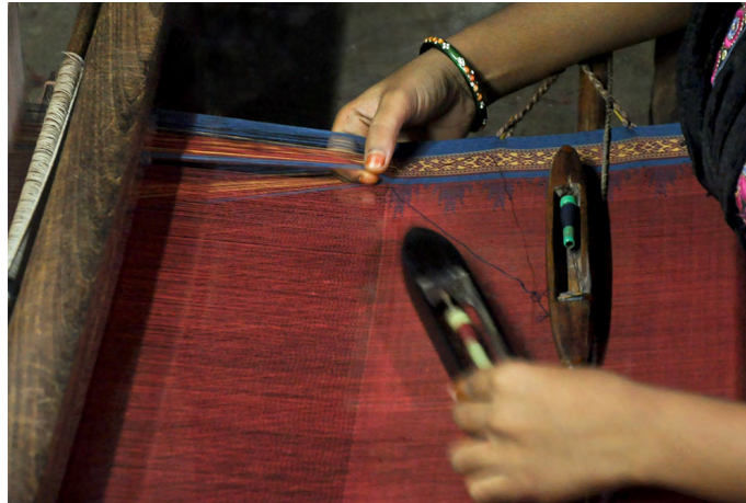
Different flying shuttles are used to make border designs.
