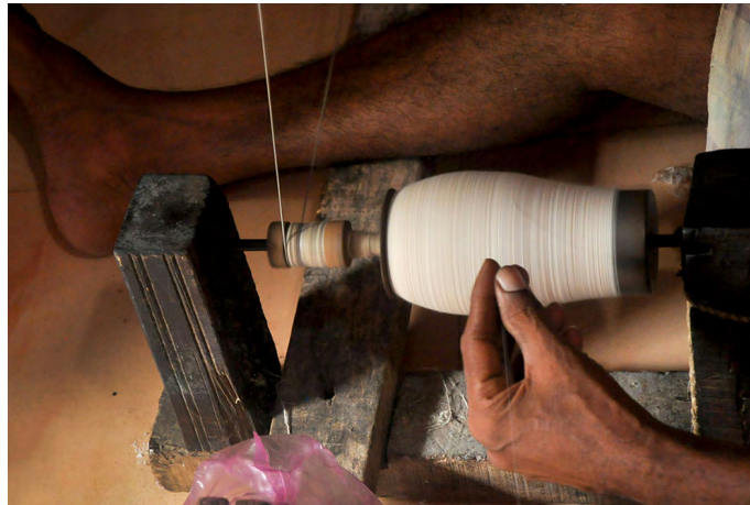
Yarns are wrapped around bobbin cone using charkha.
