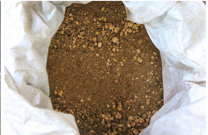
Myrobalan powder is used as a blender to obtain natural colour.
