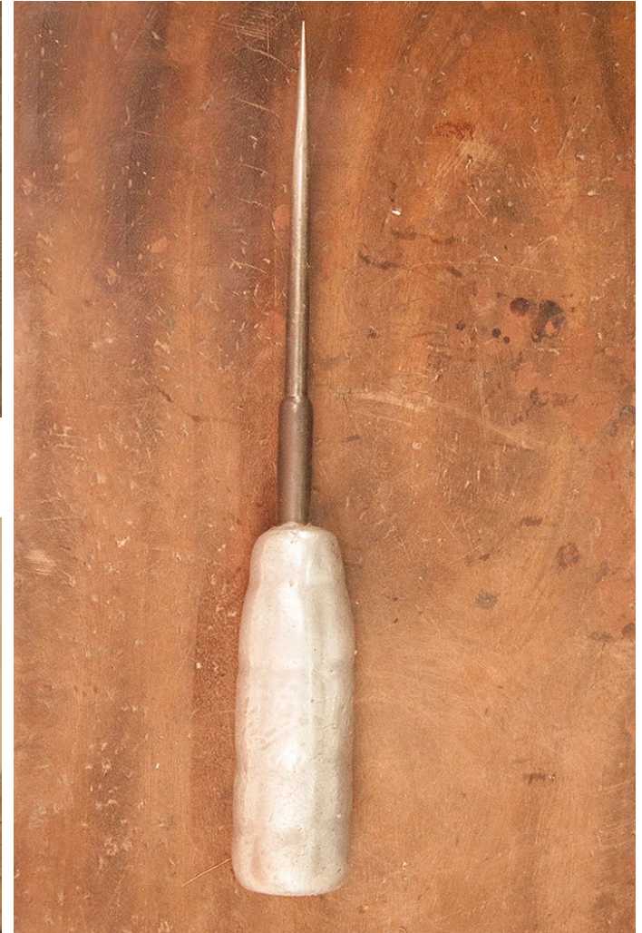
A pointed tool to make holes that helps in tieing pudi to the drum.
