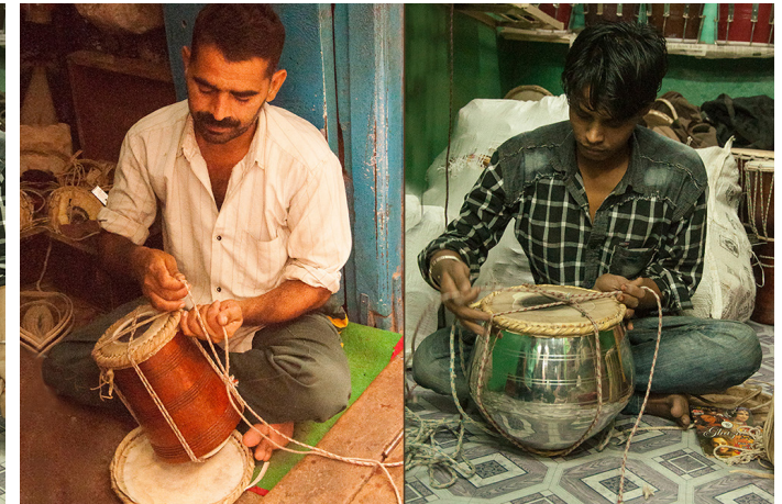
Rope is being tied to fix the drum head and the base.
