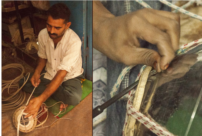
Tan (lace) is tied through the holes that pass through the drum head.
