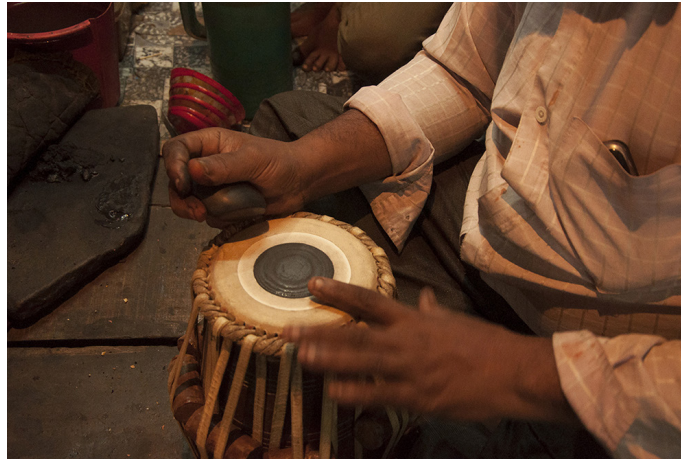
Syahi is rubbed with the stone to spread it evenly and help fine tune.
