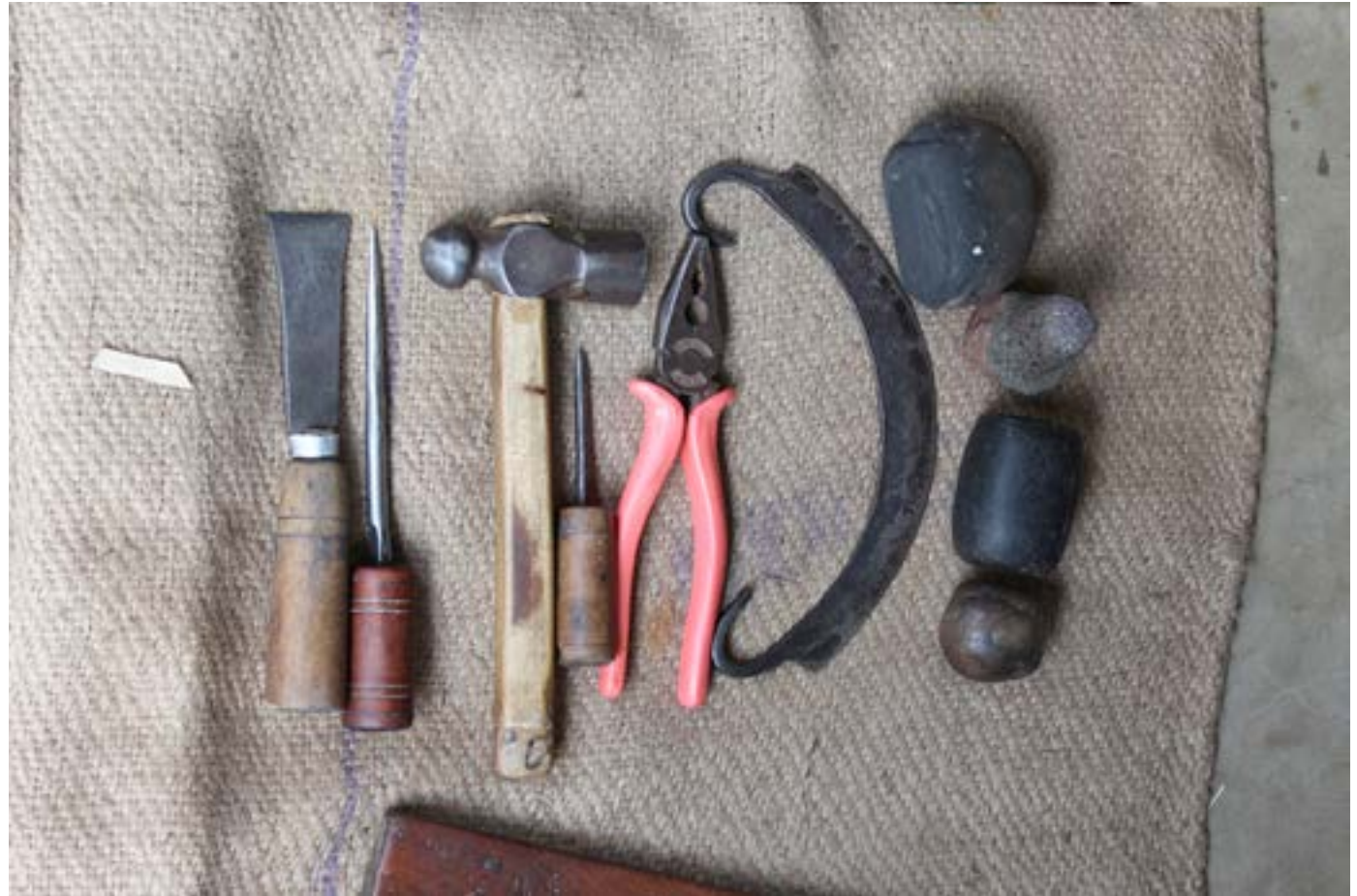
Various kinds of chisels and cutting tools are used for making Dagga.
