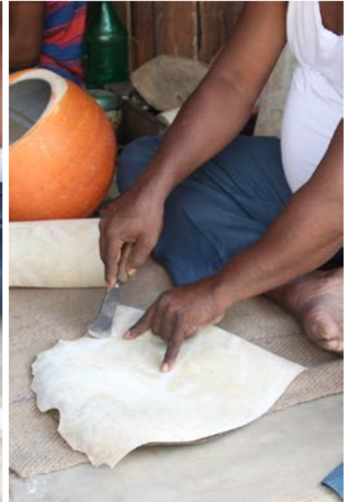
The circles are marked and then cut, and the unused sections are cut into trapezoids of varying sizes.
