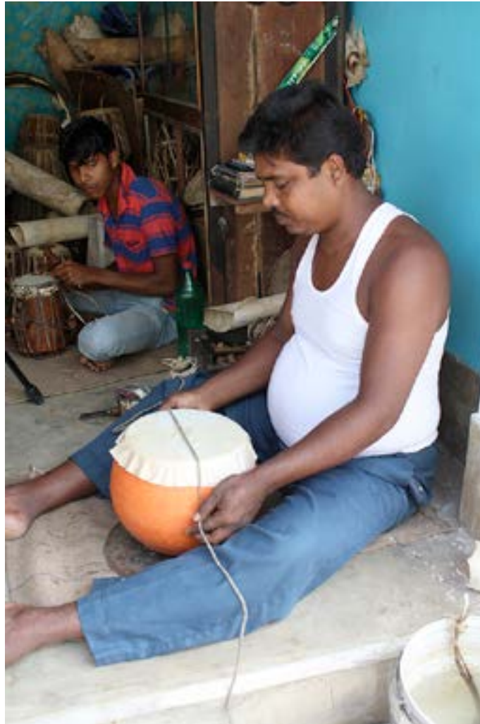
The terracotta pot and the rawhide are tied securely with the rope.
