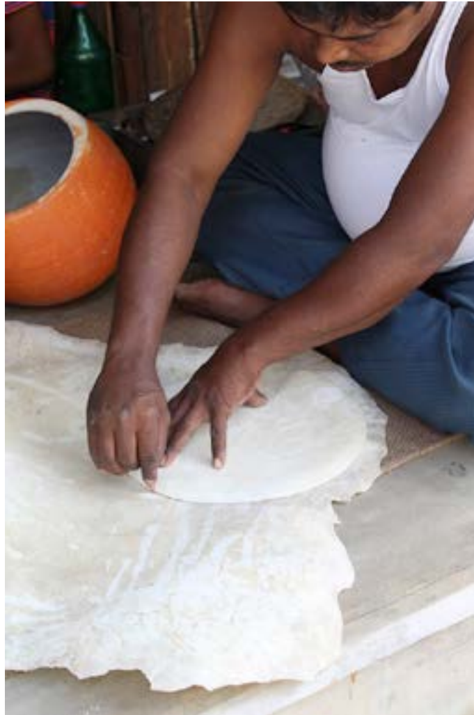
A layer of goatskin is made up of small overlapping pieces to add strength.
