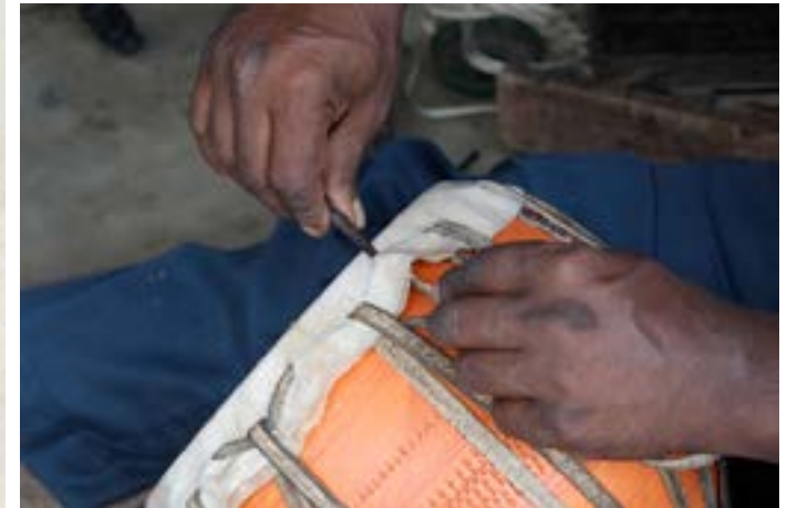
A pointed Chisel is used to pierce a hole in the leather sheet.
