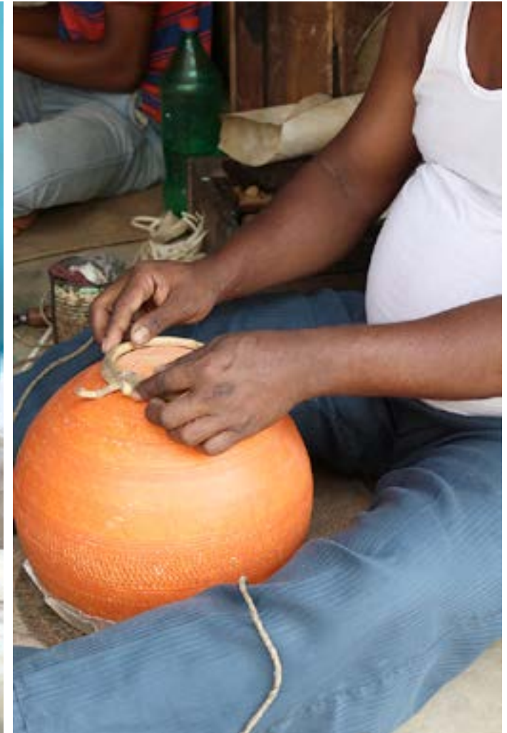
Buffalo hide is rolled and tied to the base of the terracotta pot.
