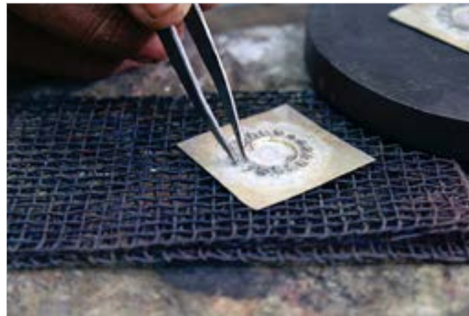
These tiny silver balls are immersed in solution and then arranged carefully in a circular form by glancing the real design.
