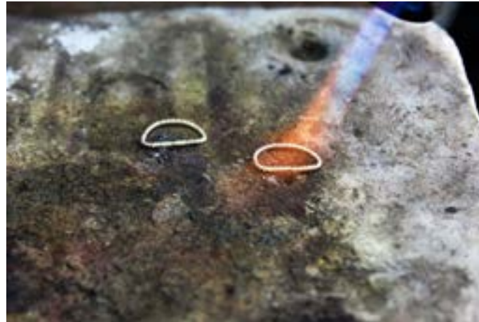
Silver ring is heated using hand gas burner.
