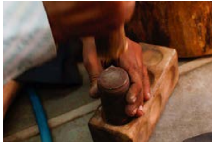
Article is being hammered to get a bulge shape.
