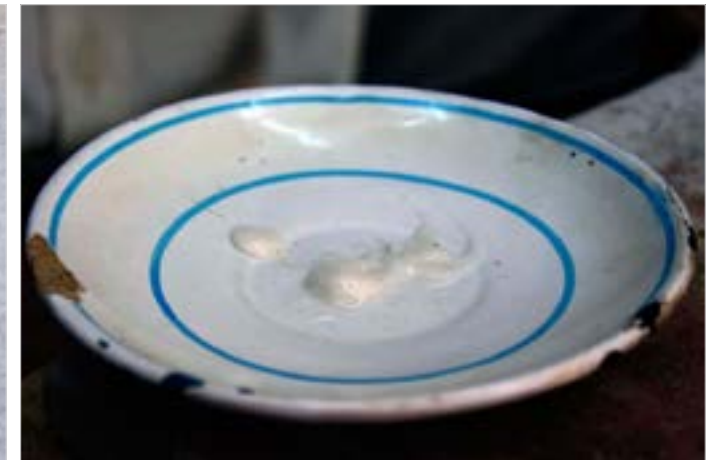
Water-soluble flux paste is used to solder the metal pieces.
