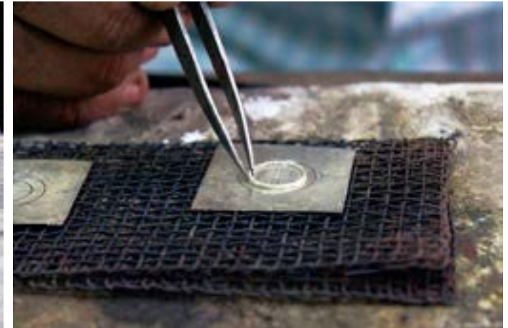
Round shaped silver ring is placed over the silver sheet by dipping the ring in a water-soluble flux paste and water.
