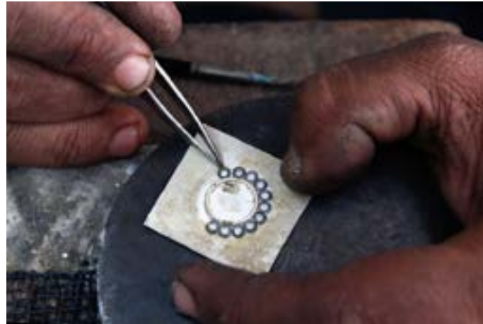
Small round shaped thin metal wires are arranged by following the actual design.
