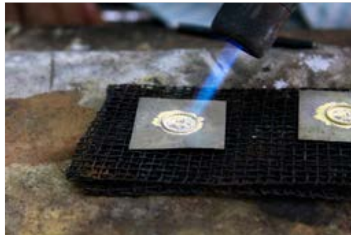
Silver ring is heated using burner so that the ring gets welded with the sheet.
