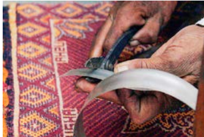
Silver sheet is cut into the required size and shape using a metal sheet cutter.
