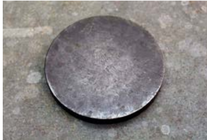
Flat solid iron surface is used while making silver jewelry.
