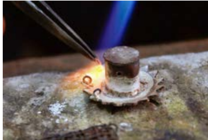
Small bells are added to the back side of the pendant and it is soldered.
