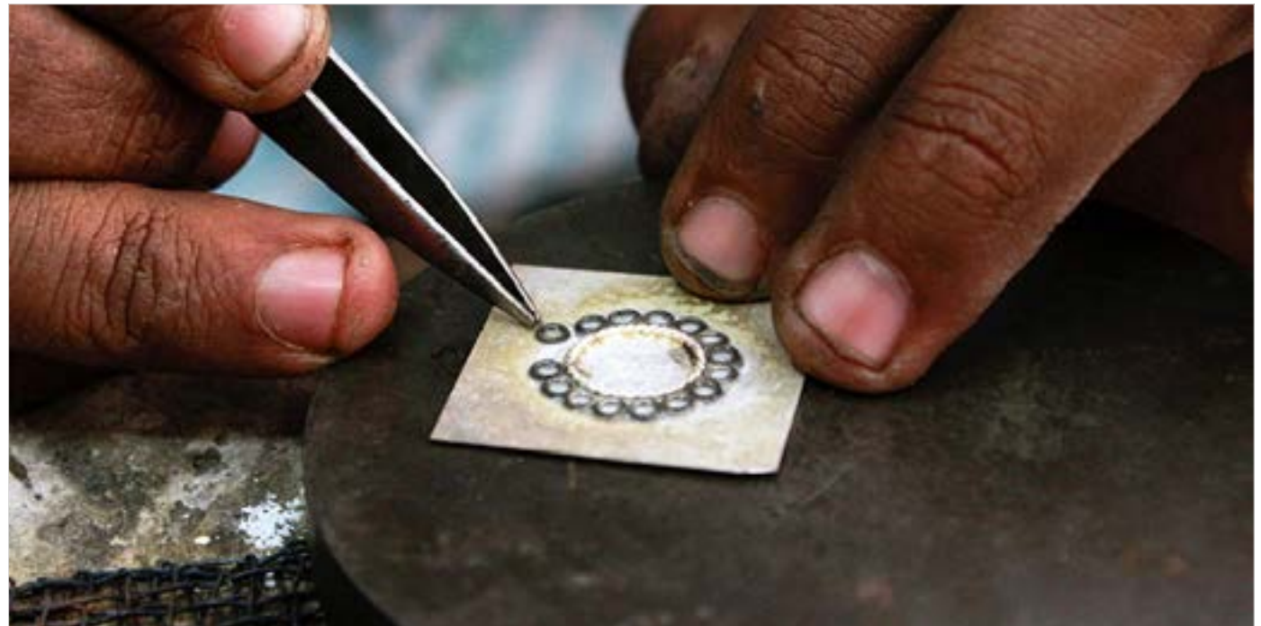
Tiny silver rings are arranged and fused using hand gas burner.
