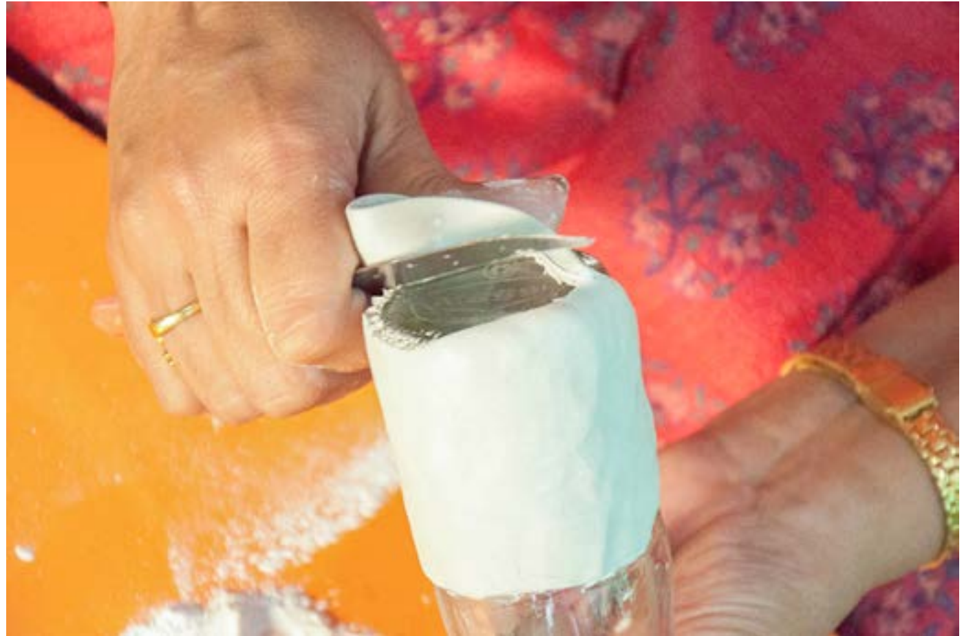
The removal of excess M-SEAL.
