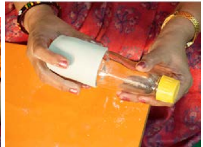
Over that M-SEAL is stuck as the base layer.
