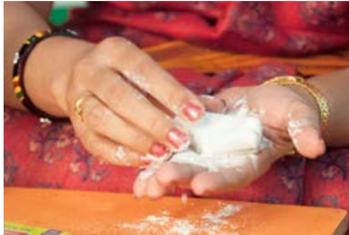
Both the M-SEAL are mixed and kneaded thoroughly.
